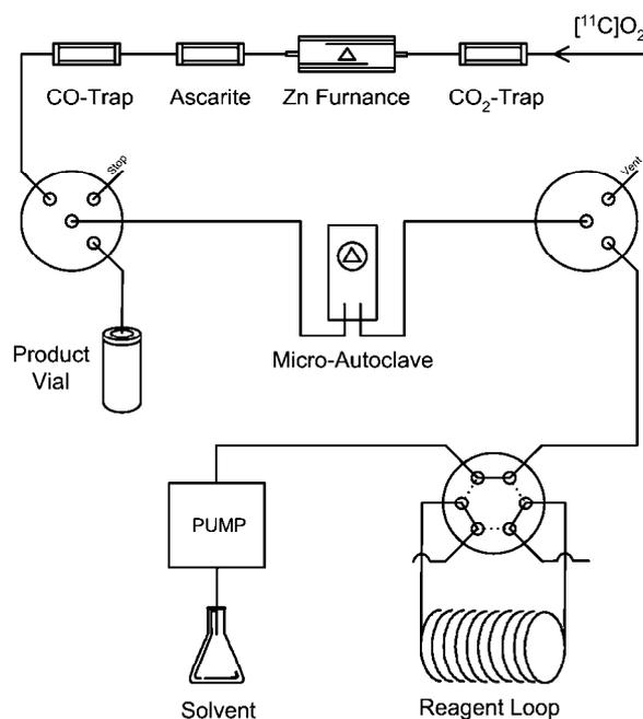
**Figure 4.** Schematic drawing of the experimental set-up used in the carbonylation reactions.
