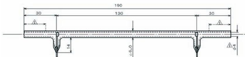
**Figure 2.** Glow discharge plasma reactor (mm). The electrodes were made of tungsten and the reactor body from quartz glass.
