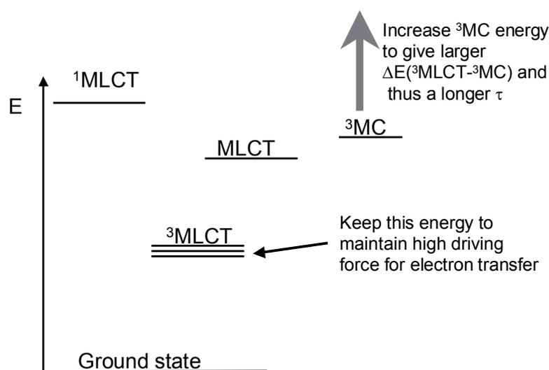
Figure 10. Description of our design strategy to extend the excited state lifetime but still maintain the excited state energy of a bis-tridentate  $\text{Ru}^{\text{II}}$ -polypyridyl complex.
