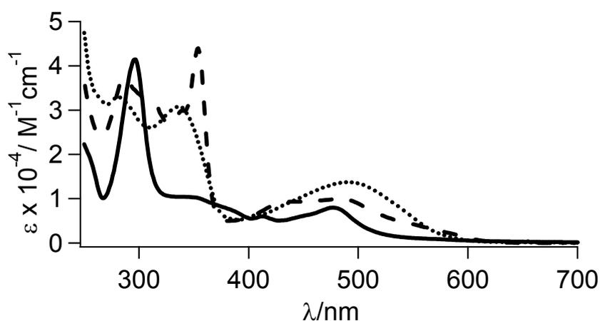
Figure 14. Absorption spectra for  $[\text{Ru}^{\text{II}}(\mathbf{1})_2]^{2+}$  (solid line),  $[\text{Ru}^{\text{II}}(\mathbf{6})_2]^{2+}$  (dashed line) and  $[\text{Ru}^{\text{II}}(\mathbf{8})_2]^{2+}$  (dotted line) in acetonitrile.
