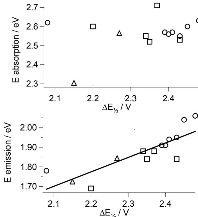
Figure 15. Upper: Correlation between absorption energy and electrochemical potentials. Lower: Correlation between emission energy and electrochemical potential. The straight line is the result of a linear fit to all data points, giving a slope of 0.74. Circles: first generation, triangles: second generation, squares: third generation.
