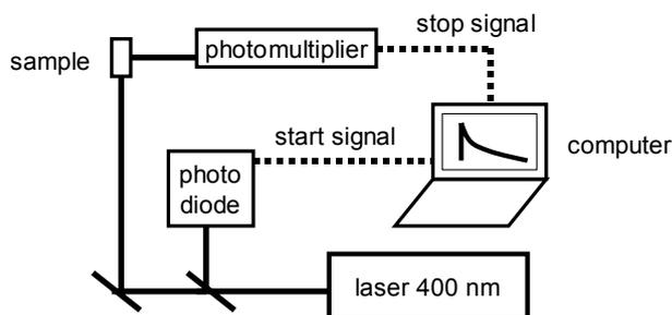
Figure 29. Schematic picture of the single photon counting experimental set up.
