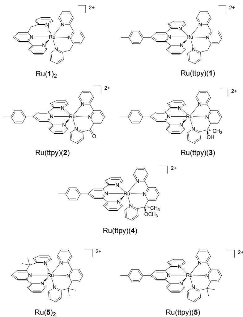
Figure 11. Structures of the complexes investigated in the first generation of photosensitizers.
