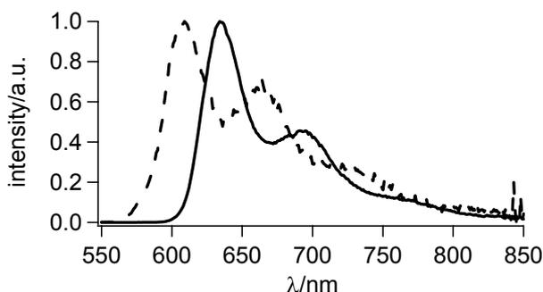
Figure 16. Normalized and detector sensitivity corrected steady state emission spectra for  $[\text{Ru}^{\text{II}}(\text{tpp})(\mathbf{1})]^{2+}$  (solid line) and  $[\text{Ru}^{\text{II}}(\mathbf{1})_2]^{2+}$  (dashed line).
