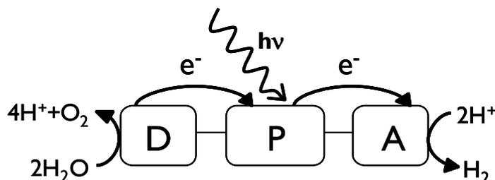
Figure 2. Schematic picture of the three necessary building blocks of an artificial photosynthetic system, where **D** denotes the electron donor capable of oxidizing water, **P** the photosensitizer collecting the sunlight and **A** the electron acceptor capable of reducing protons.
