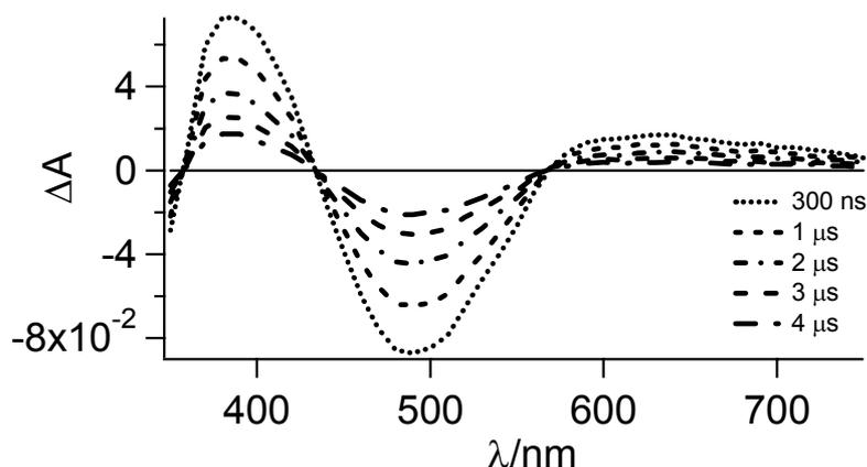
Figure 19. Transient absorption spectrum for  $[\text{Ru}^{\text{II}}(\mathbf{8})_2]^{2+}$  in deoxygenated acetonitrile solution.
