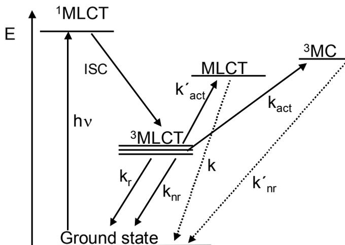
*Figure 6.* Schematic description of the excited state manifold of Ru<sup>II</sup>-polypyridyl complexes. The rate constants are denoted *k* together with a suffix indicating the type of transition.
