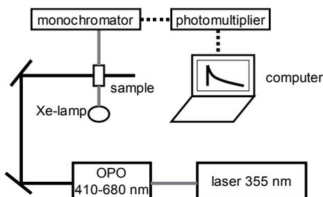
Figure 28. Schematic picture of the flash photolysis experimental set up.
