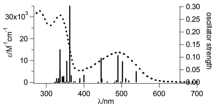
Figure 27. Comparison of experimentally obtained and TD-DFT calculated absorption spectrum for  $[\text{Ru}^{\text{II}}(\mathbf{8})_2]^{2+}$ . Dotted line: experiment, and bars: calculations.
