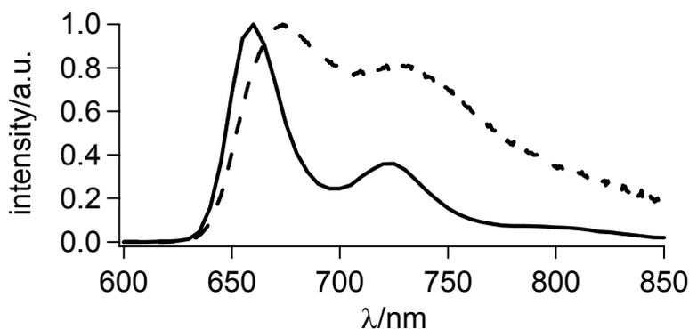
Figure 18. Normalized and detector sensitivity corrected steady state emission spectra for  $[\text{Ru}^{\text{II}}(\text{tpy})(\mathbf{8})]^{2+}$  (solid line) and  $[\text{Ru}^{\text{II}}(\mathbf{8})_2]^{2+}$  (dashed line).
