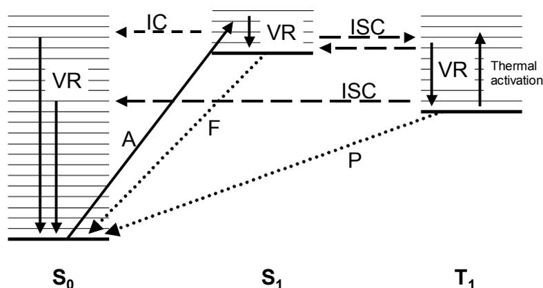
Figure 5. Jablonski diagram showing the possible radiative and nonradiative processes discussed in the text. Note that the  $S_1$  state is shown to the right for clarity reasons, not reflecting a real displacement. A denotes absorption, F fluorescence and P phosphorescence.
