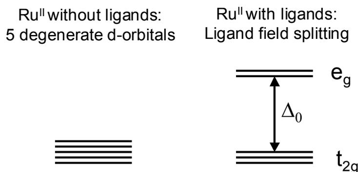
*Figure 9.* Schematic picture of the splitting between the  $t_{2g}$  and the  $e_g$  orbitals occurring when ligands are coordinated to the metal. The ligand field strength parameter  $\Delta_0$  is also indicated.
