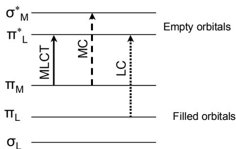
Figure 7. Schematic picture of the different absorption processes in  $\text{Ru}^{\text{II}}$ -polypyridyl complexes.
