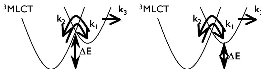
Figure 20. Schematic picture of possible activated pathways for the  $^3\text{MLCT}$  state. Left: the case where surface crossing is irreversible and  $\Delta E$  reflects the activation barrier. Right: the case where an equilibrium is established and  $\Delta E$  reflects the free energy difference between the two states, together with a possible  $\Delta E$  for  $k_3$ .
