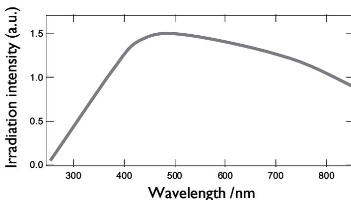
Figure 3. Schematic picture of the sun irradiation intensity distributed over wavelength.<sup>[51]</sup>
