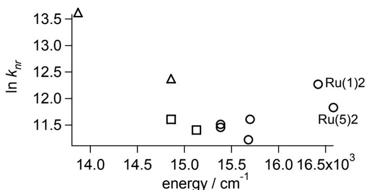
Figure 22. Correlation between the logarithm of the nonradiative rate constant at 80 K and the emission energy. Circles: first generation, triangles: second generation, and squares: third generation.
