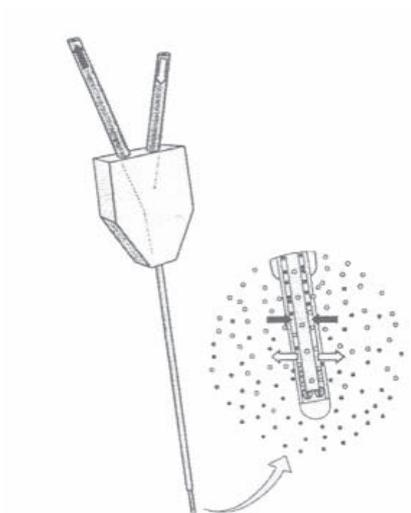
Figure 4. The principle of microdialysis. The perfusate enters through the inner cannula to the tip of the probe, where a semi permeable membrane allows exchange between the perfusate and the surrounding tissue before collected in fractions (Ungerstedt, 1991).
