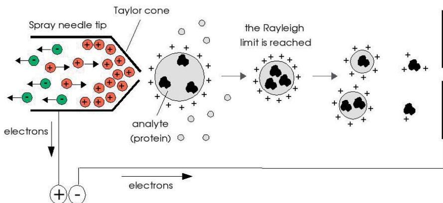
*Figure 2.3:* An illustration of the electrospray ionization process showing the evaporation and subsequent disintegration of the charged droplets, until the final production of gas phase ions.
