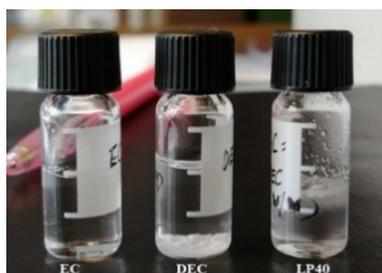
Figure 9. Solubility tests using PAN mixed with EC, DEC and LP40 solution.
