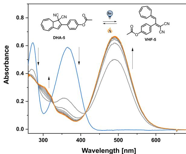
**Figure 2.** Photochemical Ring-opening reaction of **DHA-5** in DMSO (33  $\mu\text{M}$ ) upon irradiation with a 365 nm LED.
