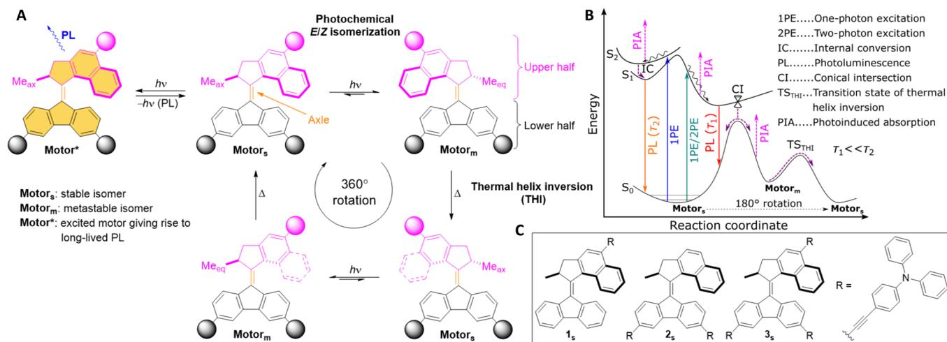
**Fig. 1. Concept and compounds used in this study.** (A) Scheme illustrating rotation and PL from a higher-lying excited-state isomer of a second-generation molecular motor. (B) Conceptual potential energy diagram illustrating the mode of operation of the molecular motors described in this study capable of performing rotation and undergoing relaxation via PL. (C) Compounds used in this study.
