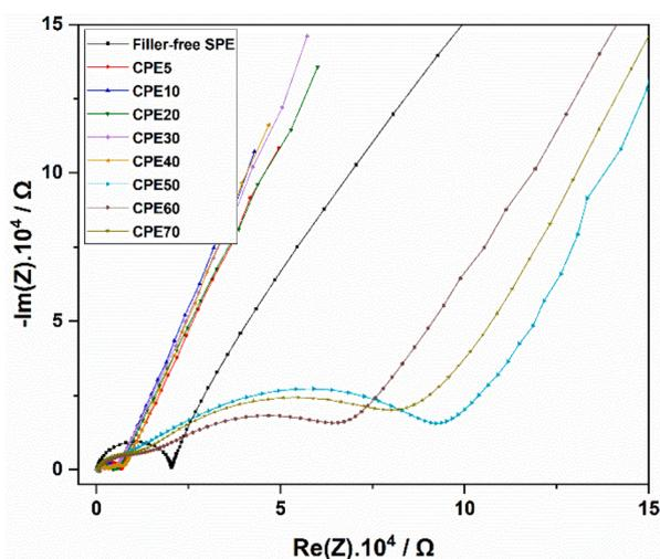
Fig. 3. Electrochemical impedance spectroscopy measurements of SPE and CPE electrolytes from 7 MHz to 100 mHz: Nyquist plot of SPE and CPEs at 60 °C.
