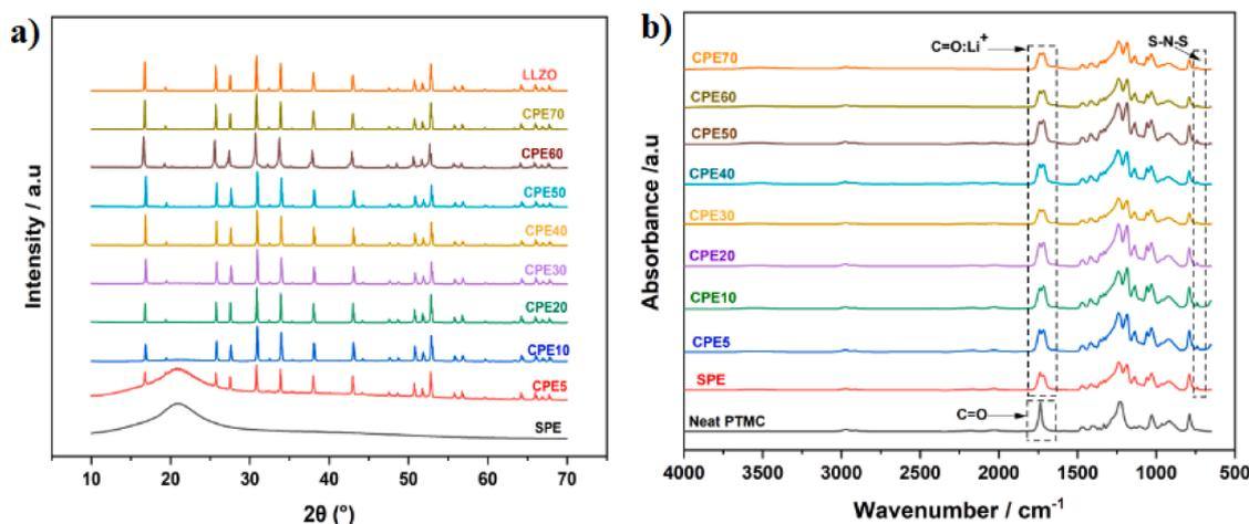
Fig. 2. (a) X-ray diffraction patterns of filler-free solid polymer electrolyte (SPE), composite electrolytes (CPEs), and pristine LLZO powder; (b) FTIR spectra of SPE, CPEs, and pristine PTMC polymer.
