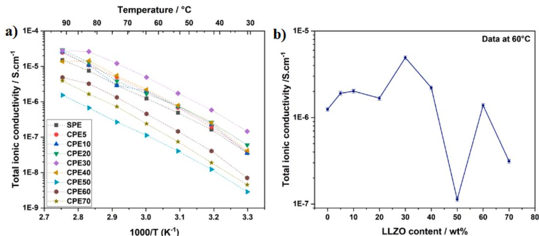
Fig. 4. (a) Arrhenius-type plots of the total ionic conductivity of SPE and CPEs from 30 to 90 °C within the entire range of LLZO concentration; (b) Li-ion conductivity as function of the ceramic LLZO concentration at 60 °C. Standard error of the mean is represented as error bars.
