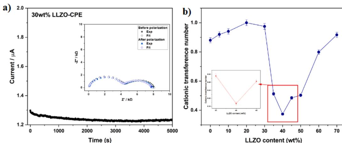
**Fig. 6.** (a) Chronoamperometric response of a Li/CPE30/Li symmetrical cell at 60 °C. Inset: Nyquist plot before and after polarization; (b) Variation of the cationic transference number as function of LLZO ceramic concentration. Inset:  $T_+$  variation from 35 to 45 wt% of LLZO. Standard error of the mean is represented as error bars.
