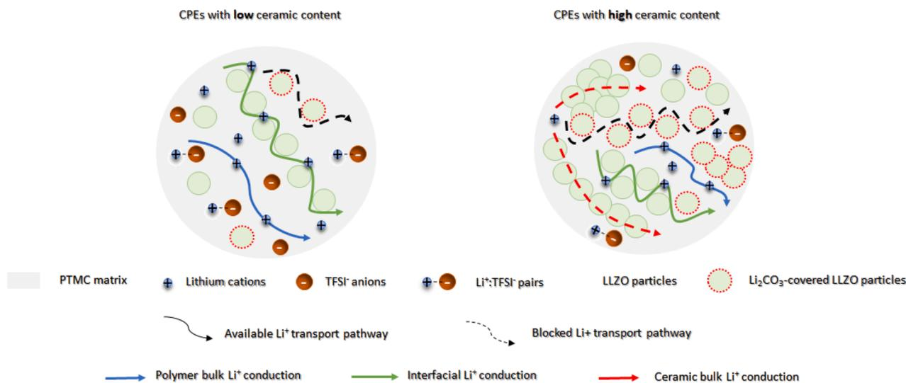
Fig. 8. Schematic representation of different possible Li-ion transport pathways in PTMC-LLZO composite electrolytes for low and high ceramic concentration. Straight and dashed lines represent the conductive and restricted ionic transport routes, respectively.
