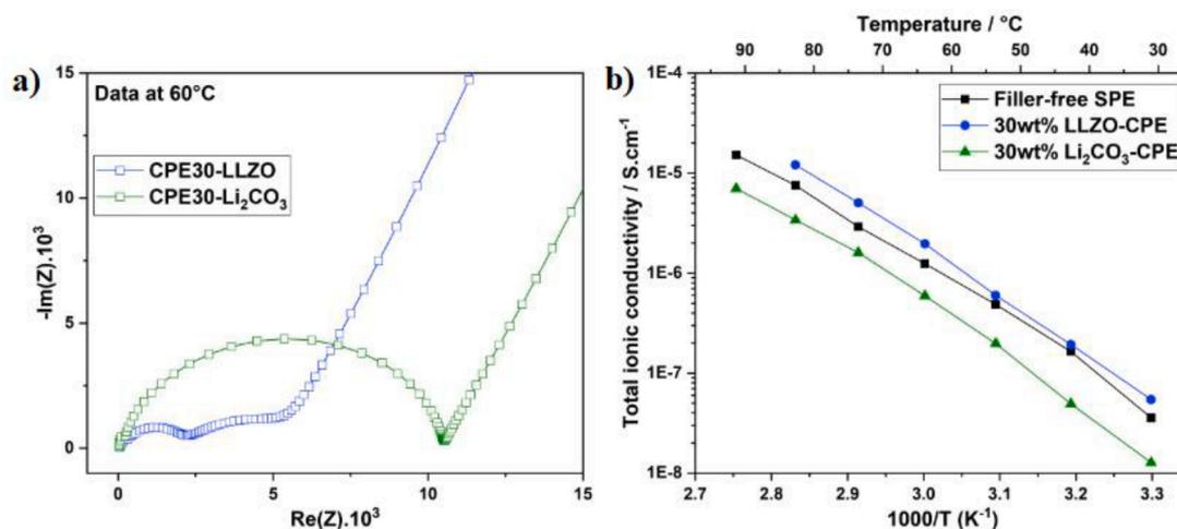
Fig. 7. (a) Nyquist plot of the composite electrolytes with 30 wt% of LLZO and  $\text{Li}_2\text{CO}_3$  at 60 °C; (b) temperature-dependent variation of the total ionic conductivity of SPE, and CPEs with either 30 wt% of LLZO and  $\text{Li}_2\text{CO}_3$ .
