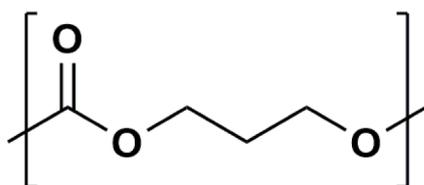
Fig. 1. Structure of poly(trimethylene carbonate).
