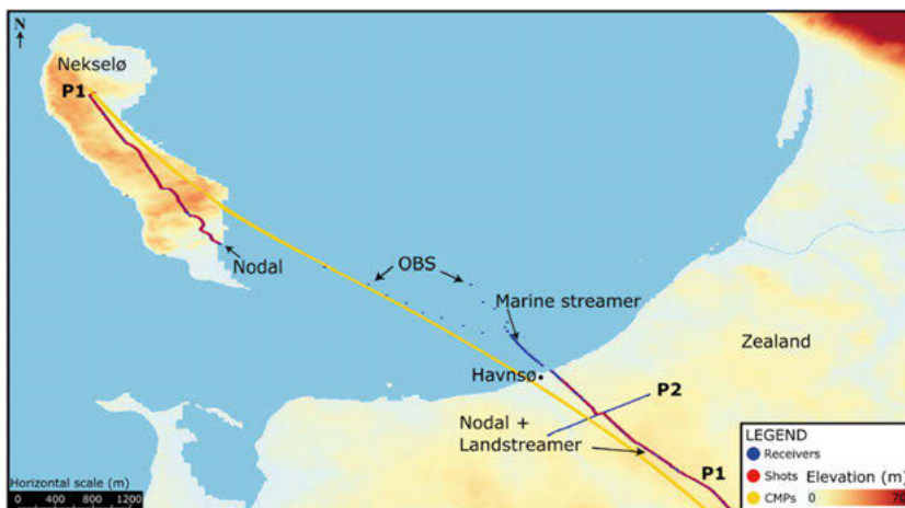
Figure 3.2. The marine channel acquisition setup on the northern part of profile 1 (P1) between the Havnsø town and Nekselø island. In red are the shot positions; in blue are the receiver positions with labels indicating the type of sensors; and in yellow are the adopted CMP positions for the final stack. The offshore areas are shown in light blue.
