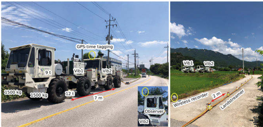
Figure 3.1. Field photos, from South Korea campaign, exemplifying the seismic source and receivers of the dual-element acquisition system.
