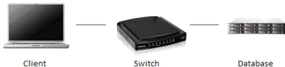
Figure 1.5.1. The image shows the design of the test environment. The client is connected to the server through a Local Area Network.
