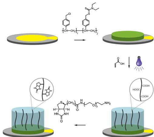
**Fig. 1** Fabrication of biotin-functionalized pAAc sensor. Gold-plated QCM crystals were first coated with the photoreactive copolymer PVBD<sub>501</sub>, which was subsequently subjected to poly(acrylic acid) brush formation under UV irradiation. Final coupling of (+)-biotinyl 3,6,9-trioxaundecanediamine to the carboxylic acid groups yielded functionalized QCM sensor surfaces of three-dimensional character.
