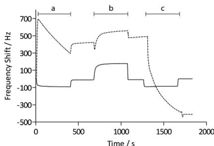
**Fig. 2** Frequency responses of the surface derivatization process at the pAAc surface (---), and the carboxyl-terminated SAM surface (—), respectively. Injections for activation by EDC/sulfo-NHS (a); functionalization with (+)-biotinyl 3,6,9-trioxaundecanediamine (b); and deactivation by ethanolamine (c), are indicated in the graph.
