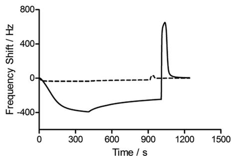
**Fig. 4** Frequency responses of protein binding and sensor surface regeneration. Anti-biotin  $F_{ab}$  binding to biotin-derivatized pAAc surface (—); anti-biotin  $F_{ab}$  binding to biotin-derivatized carboxyl-terminated SAM surface (---). Sample concentrations:  $25 \mu\text{g mL}^{-1}$ ; flow rate:  $25 \mu\text{L min}^{-1}$ . Surfaces were regenerated with glycine (10 mM,  $pH = 1.5$ ).
