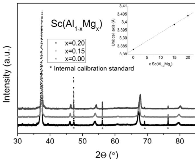
Figure 6.9. XRD pattern of Sc(Al<sub>1-x</sub>Mg<sub>x</sub>), x ≤ 0.20. From the top: x = 0, 0.15, 0.20. Silicon is used as internal calibration standard. The inset shows the unit cell axis as a function of magnesium content.
