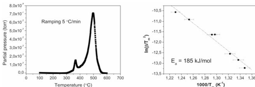
Figure 6.7. Left: TDS pattern of hydrogenated  $\text{ScAl}_{0.8}\text{Mg}_{0.2}$ . Right: Kissinger plot of hydrogenated  $\text{ScAl}_{0.8}\text{Mg}_{0.2}$ . The error bars indicate an estimated error of  $\pm 5$  °C.
