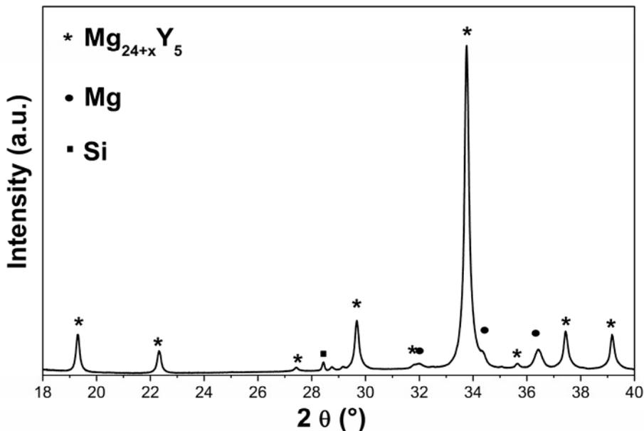
Figure 5.2. XRD pattern of the Mg-Y-Ti alloy. Si was used as internal calibration standard.
