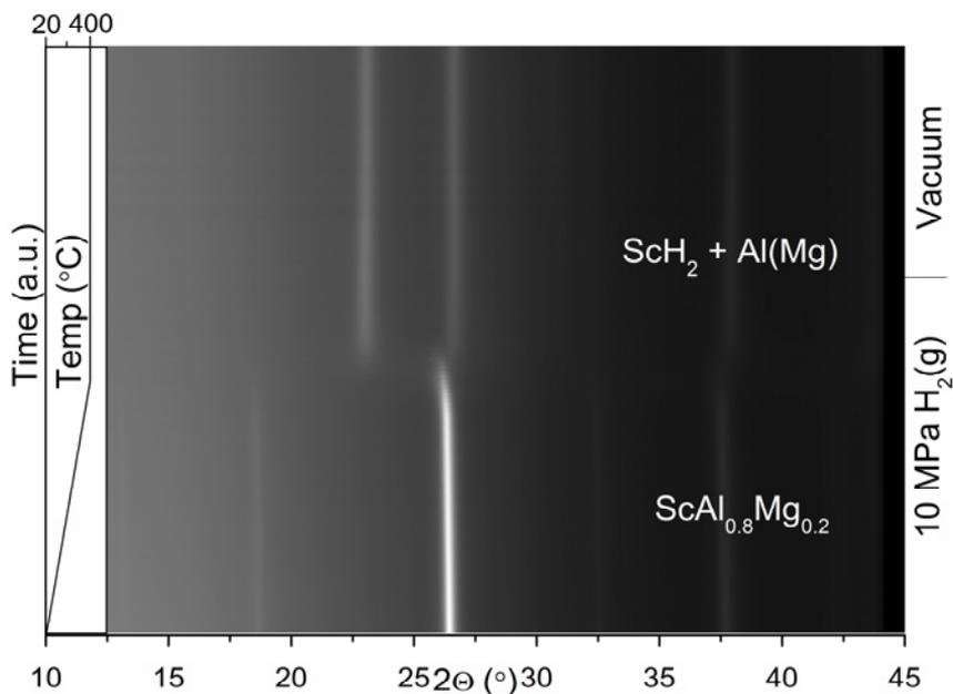
Figure 6.4. Hydrogen absorption in  $\text{ScAl}_{0.8}\text{Mg}_{0.2}$  investigated with *in situ* SR-XRD.
