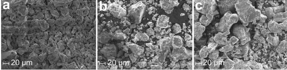
Figure 6.12. a, SEM images of the hydrogenated sample ( $\text{Sc}(\text{Al}_{1-x}\text{Mg}_x)$ ,  $x = 0.20$ ). b, Desorbed sample ( $x = 0.20$ ). c, Hydrogenated sample after six cycles ( $x = 0.0$ ). Magnification 1000 x.
