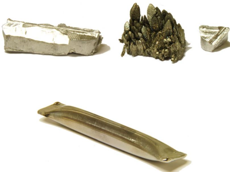
Figure 4.1. Upper part from the left: Pieces of aluminium, scandium and magnesium. Lower part: A sealed tantalum tube.
