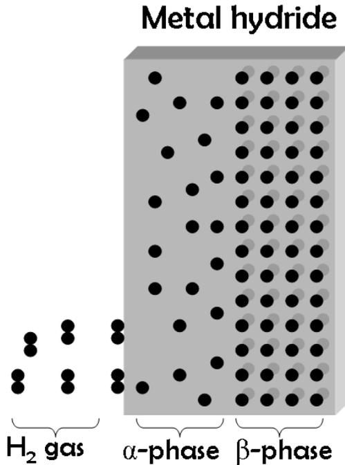
Figure 3.2. Schematic image of hydrogen in a metal. The solid solution  $\alpha$ -phase and the hydride  $\beta$ -phase.
