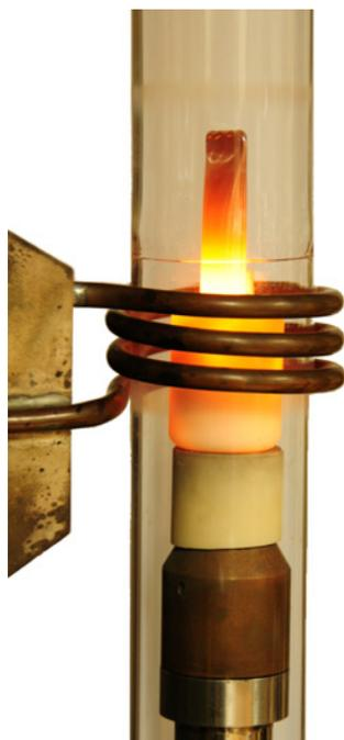
Figure 4.2. Synthesis in the induction furnace.
