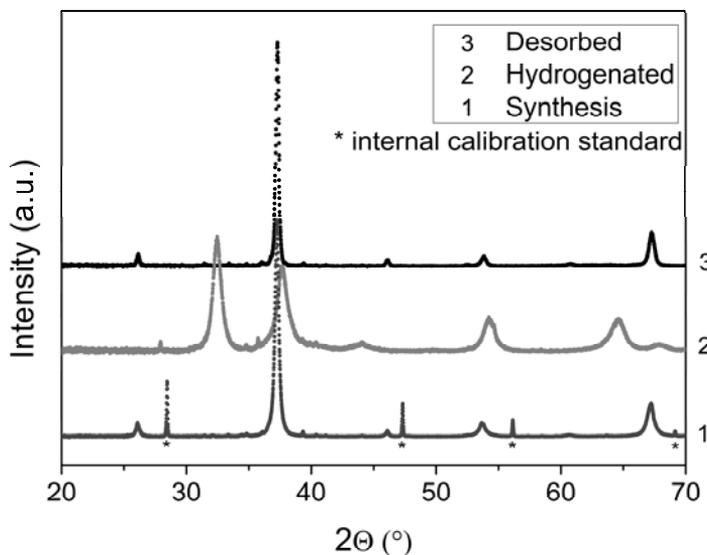
Figure 6.8. XRD of  $\text{ScAl}_{0.8}\text{Mg}_{0.2}$  after synthesis, hydrogenation and desorption. Si is used as internal calibration standard.
