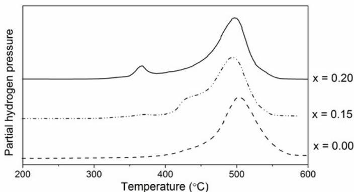
Figure 6.10. Thermal desorption spectra of hydrogenated  $\text{Sc}(\text{Al}_{1-x}\text{Mg}_x)$  for  $x = 0$ , 0.15 and 0.20, recorded for the first absorption/desorption cycle. The heating rate was  $5^\circ\text{C}/\text{min}$ .
