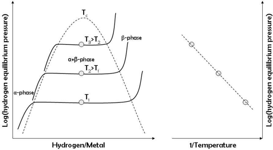
Figure 4.4. Schematic image of a pressure-composition-temperature plot and a Van't Hoff plot.
