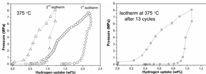
Figure 5.7. PCT of YMgGa, measured at 375 °C. Left: first and second isotherm. Right: Isotherm after 13 cycles.
