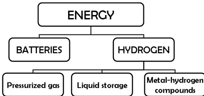
Figure 1.2. Family tree of two different ways to store energy for vehicular applications.
