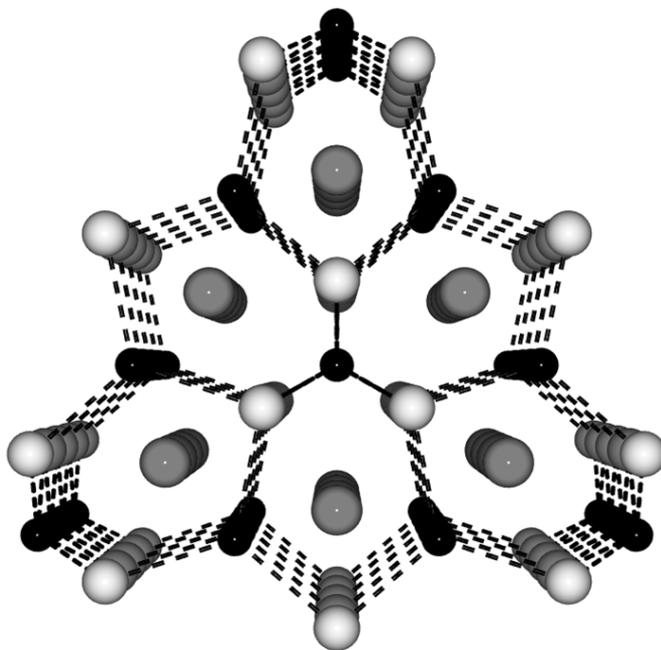
Figure 5.4. YMgGa structure along the c-axis. Mg, Ga and Y are light gray, black and dark gray respectively.
