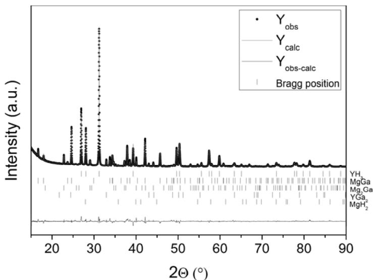
Figure 5.6. XRD pattern of YMgGa, hydrogenated at 6 MPa and 375 °C.
