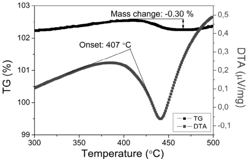
Figure 5.9. DTA/TG on hydrogenated  $\text{Mg}_3\text{Y}_2\text{Zn}_3$ .
