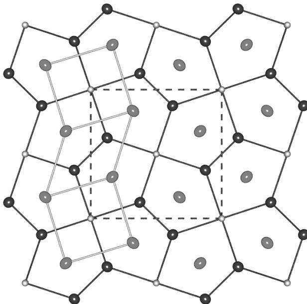
Figure 6.2. The crystal structure of  $\text{Sc}_2\text{MgGa}_2$ , along the  $c$ -axis. Sc, Mg and Ga atoms are grey, white and black respectively.
