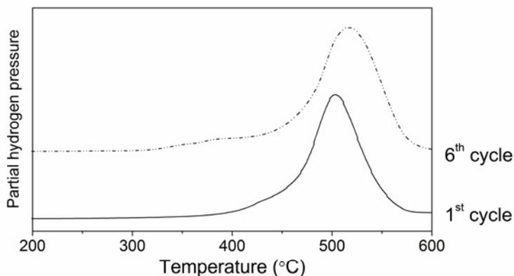
Figure 6.11. Thermal desorption spectra of  $\text{Sc}(\text{Al}_{1-x}\text{Mg}_x)$  for  $x = 0.0$ , recorded during the first and sixth desorption cycle.
