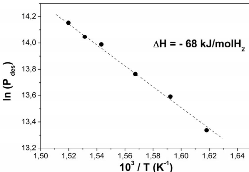
Figure 5.3. Van't Hoff plot of the hydrogen desorption from the hydrogenated Mg-Y-Ti alloy.
