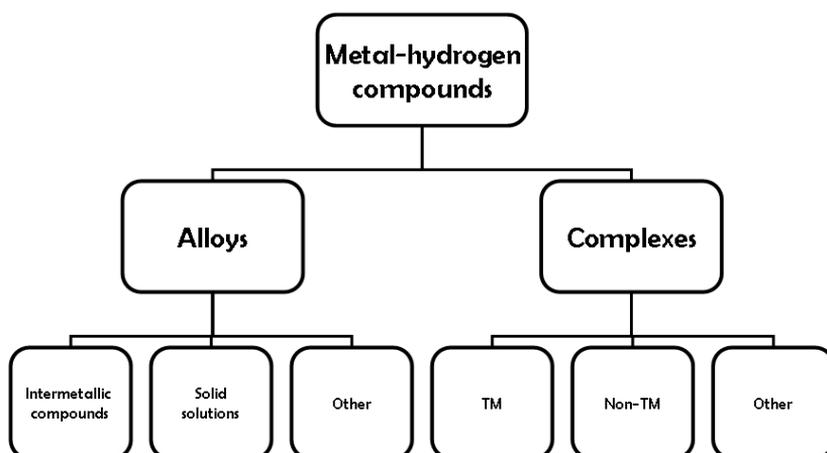
Figure 3.1. Family tree of metal hydrides, as described by Sandrock<sup>11</sup>.
