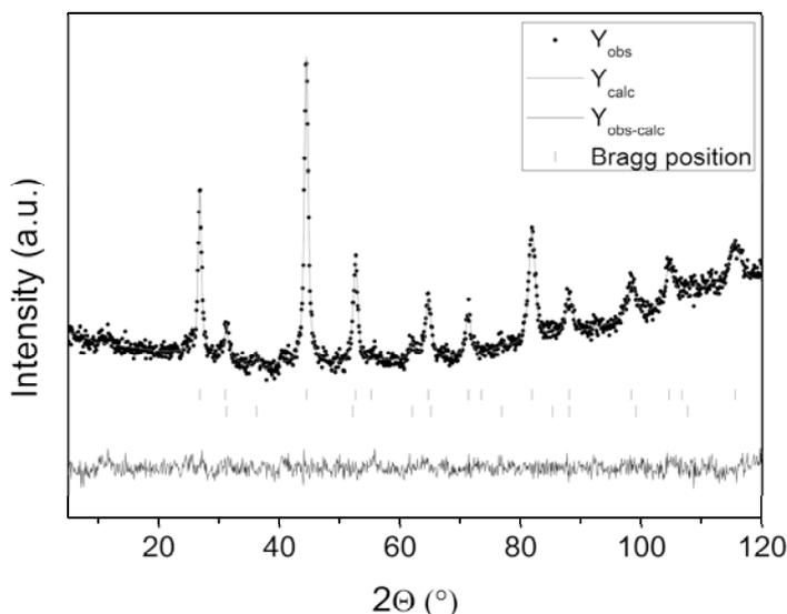
Figure 6.6. NPD pattern of deuterated  $\text{ScAl}_{0.8}\text{Mg}_{0.2}$ . The upper and lower ticks marks the Bragg positions of  $\text{ScD}_2$  and  $\text{Al}(\text{Mg})$  respectively.
