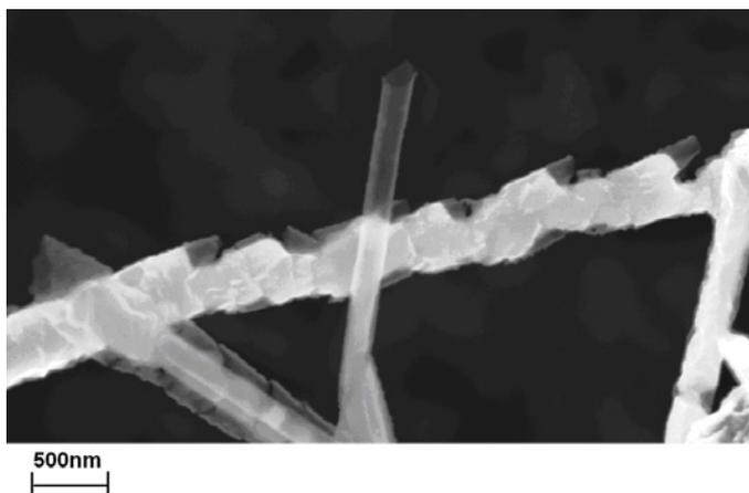
Figure 5.1. SEM image of desorbed  $\text{Mg}_{24}\text{Y}_5\text{-H}$  showing carved magnesium tubes.
