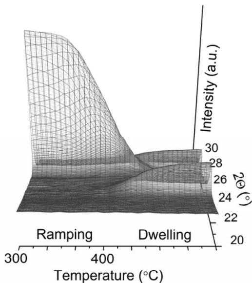
Figure 6.5. *In situ* SR-XRD data showing the decomposition from  $\text{ScAl}_{0.8}\text{Mg}_{0.2}$  to  $\text{ScH}_2$  and  $\text{Al}(\text{Mg})$ .
