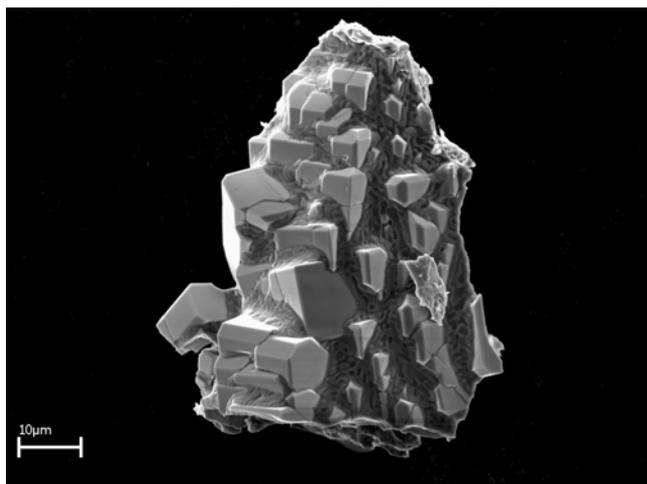
Figure 6.1. SEM image of a sample with the overall composition  $\text{ScMg}_4\text{Ga}$ . Crystals of  $\text{Sc}_2\text{MgGa}_2$  are shown in the matrix.
