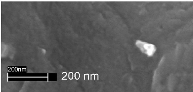
Figure 6.13. High-resolution SEM image of the hydrogenated sample ( $\text{Sc}(\text{Al}_{1-x}\text{Mg}_x)$ ,  $x = 0.20$ ). Magnification 380 kx.
