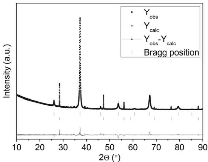
Figure 6.3 XRD pattern of  $\text{ScAl}_{0.8}\text{Mg}_{0.2}$ . The lower phase is silicon, used as an internal calibration standard.
