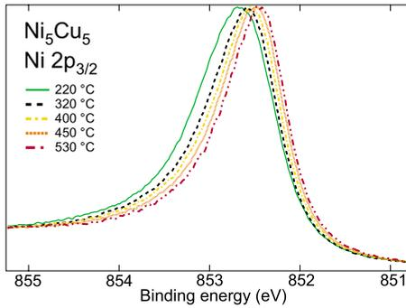
FIG. 4. (Color online) The Ni  $2p_{3/2}$  photoelectron spectra of  $Ni_5Cu_5$  measured using 2010 eV photon energy.
