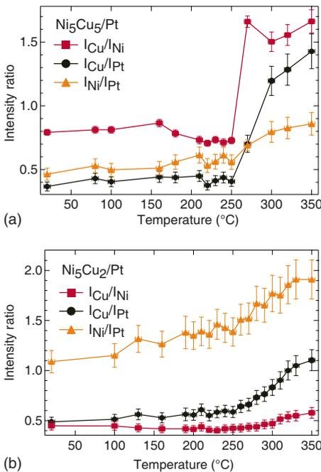
FIG. 5. (Color online) Intensity ratios between Cu  $2p$ , Ni  $2p$ , and Pt  $4f$  corelevels of  $Ni_5Cu_5/Pt$  (a) and  $Ni_5Cu_2/Pt$  (b).
