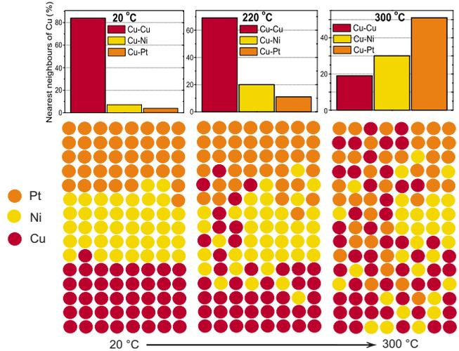
FIG. 9. (Color online) Schematic illustration of intermixing and alloying of Ni/Cu multilayers and Pt cap as a function of temperature. The changes in the chemical environment are described by histograms that are based on the two-peak-fit models of Ni<sub>5</sub>Cu<sub>5</sub>/Pt and Ni<sub>5</sub>Cu<sub>5</sub>.
