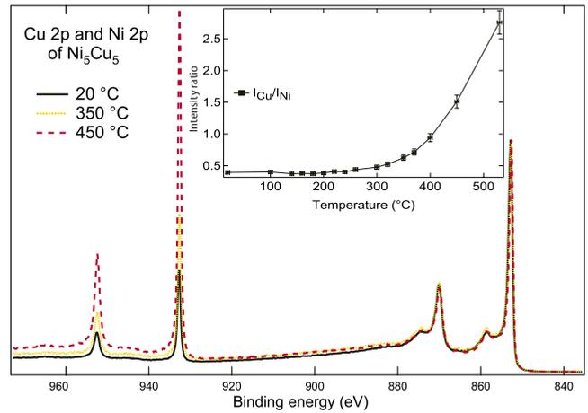
FIG. 6. (Color online) The intensity ratio of Cu  $2p$  and Ni  $2p$  photoelectron spectra measured at different temperatures using 2010 eV photon energy. The spectra are normalized to a common background before the Ni  $2p$  level. The increased intensity of Cu  $2p$  relative to the intensity of Ni  $2p$  as a function of heating temperature is due to segregation of Cu.
