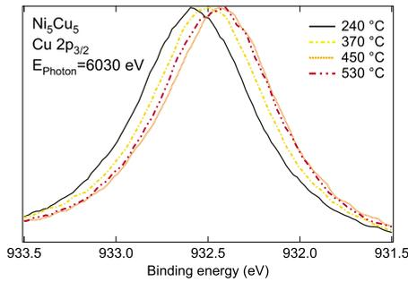
FIG. 7. (Color online) The Cu  $2p_{3/2}$  photoelectron spectra of  $\text{Ni}_5\text{Cu}_5$  measured using 6030 eV photon energy.
