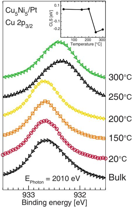
FIG. 1. (Color online) The Cu  $2p_{3/2}$  photoemission spectra of Pt capped  $\text{Ni}_5\text{Cu}_5$  measured using 2010 eV photon energy. A reference spectrum of bulk Cu (100 ML Cu) is included. The inset presents the Cu  $2p_{3/2}$  CLS as a function of temperature.
