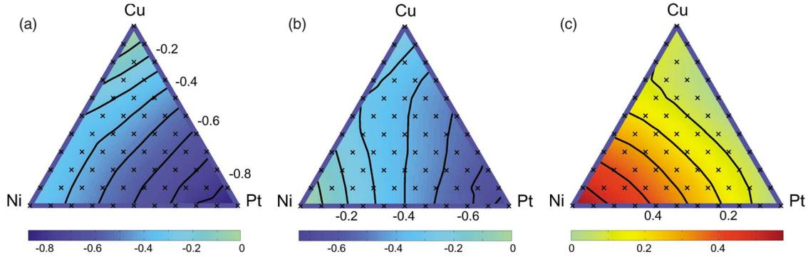
FIG. 3. (Color online) The theoretical core-level shifts of (a) Cu and (b) Ni  $2p_{3/2}$  and (c) Pt  $4f_{5/2}$  in fcc disordered ternary CuNiPt alloys are shown above. For clarity, the small circles mark incremental differences in 10 at. %. Isolines are plotted in steps of 0.1 eV over the alloy compositions. Note that the sides of the triangles correspond to the respective binary alloys.
