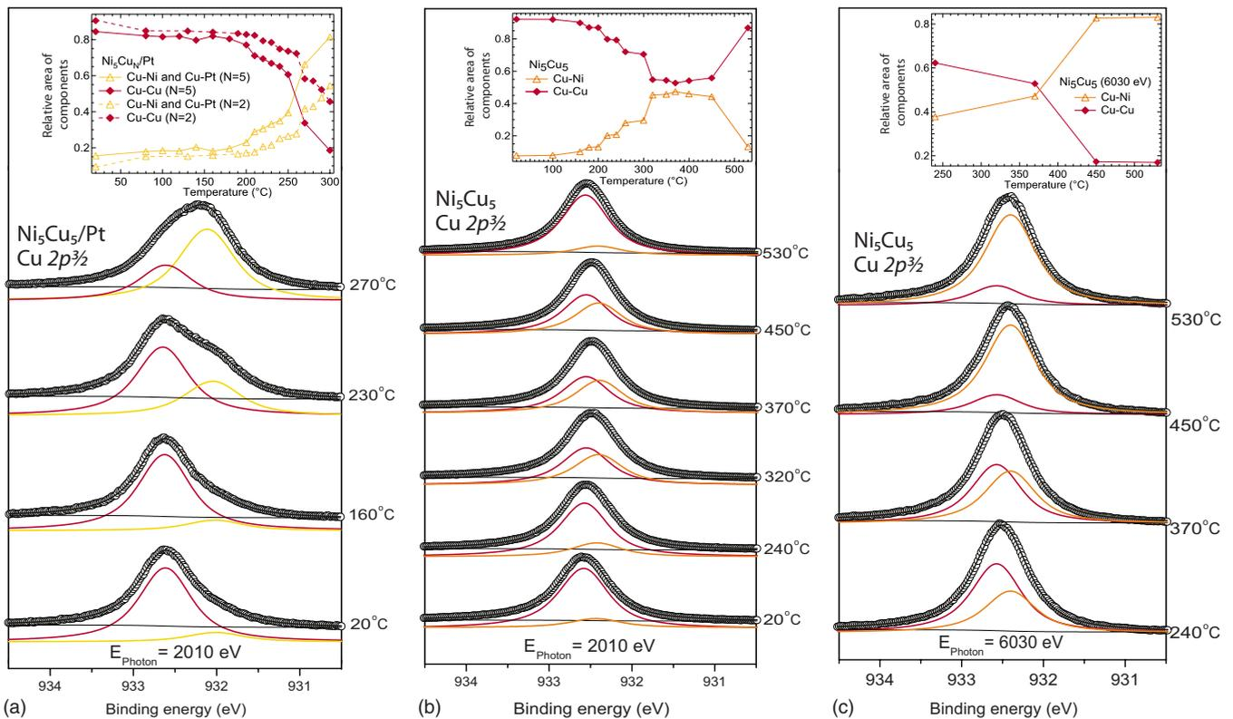
FIG. 8. (Color online) A two-peak-fit model of Cu  $2p_{3/2}$  photoelectron spectra of  $\text{Ni}_5\text{Cu}_5/\text{Pt}$  and  $\text{Ni}_5\text{Cu}_5$  at photon energy 2010 eV (a and b, respectively) and  $\text{Ni}_5\text{Cu}_5$  at photon energy 6030 eV (c). The insets show how the intensity ratio of the two components in the two-peak-fit model of  $\text{Ni}_5\text{Cu}_5/\text{Pt}$ ,  $\text{Ni}_5\text{Cu}_2/\text{Pt}$  and  $\text{Ni}_5\text{Cu}_5$  changes as a function of temperature.
