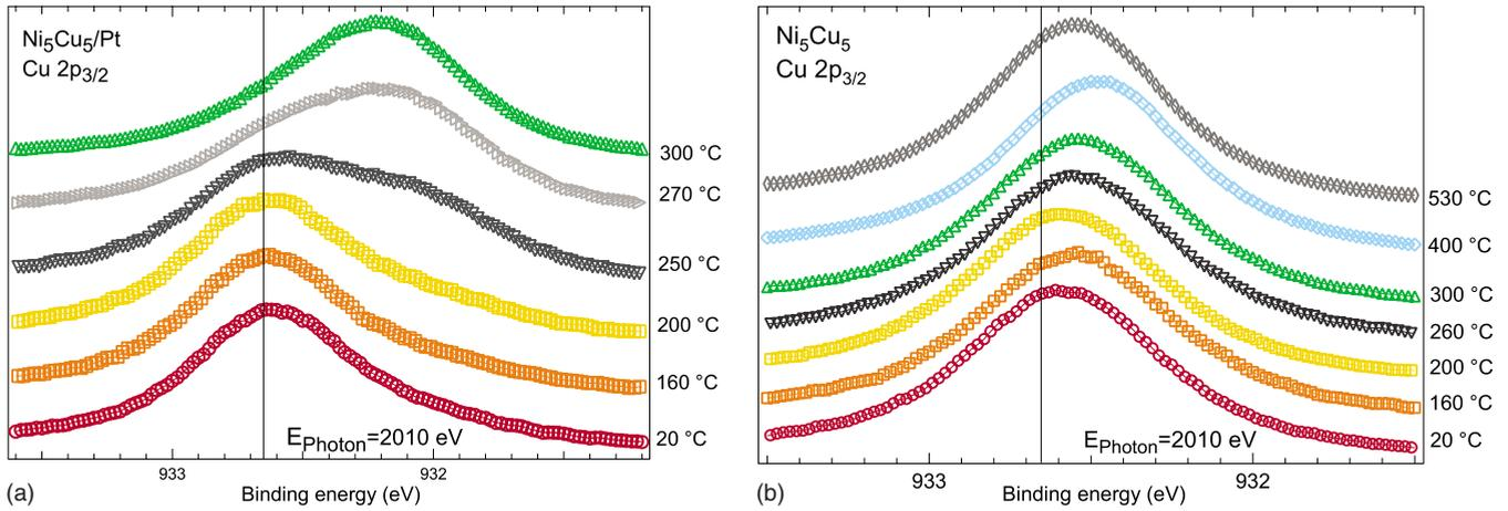
FIG. 2. (Color online) The Cu  $2p_{3/2}$  photoelectron spectra of  $\text{Ni}_5\text{Cu}_5/\text{Pt}$  (a) and  $\text{Ni}_5\text{Cu}_5$  (b) measured using 2010 eV photon energy. The black line corresponds the binding energy of bulk Cu  $2p_{3/2}$ .
