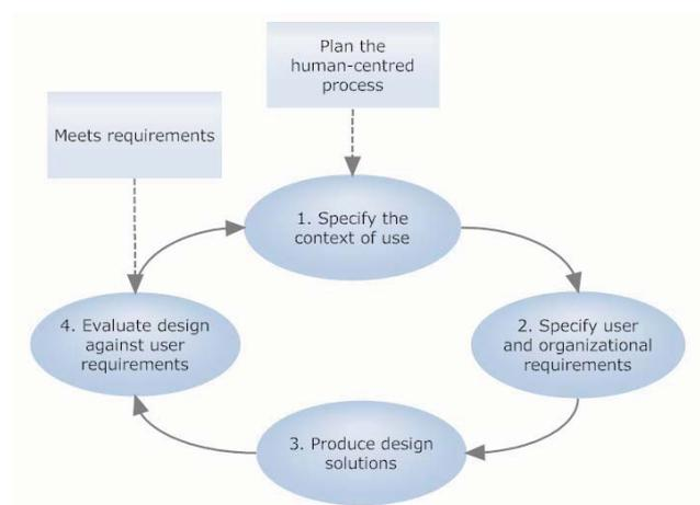
Figure 1: Human-centred design process according to ISO 13407
