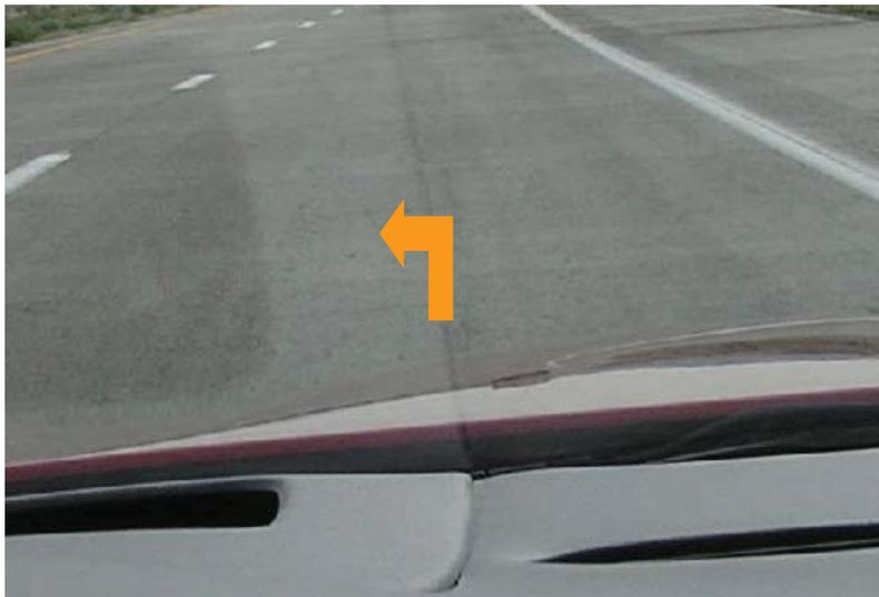
Figure 11: Concept C1 - Different gap safety levels displayed as changing arrow colours on the HUD.
