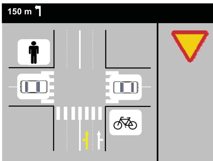
Figure 9: Combination of concept A2 and B2 - Information about an intersection and about other road users.
