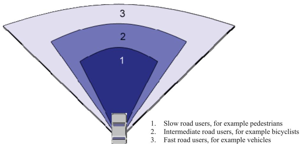
*Figure 10: Illustration of potential areas of interest for a driver driving straight ahead*
