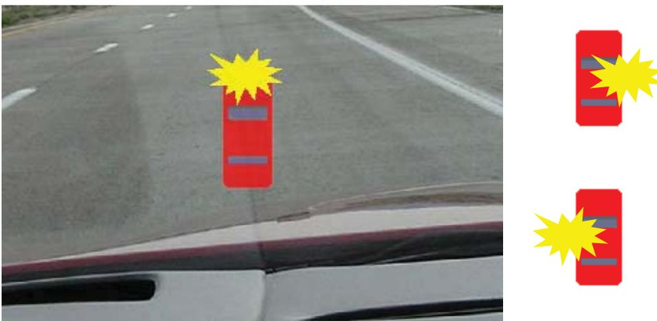
Figure 14: Visual concept for D2 - A car with a crash symbol indicating the direction of the hazard.
