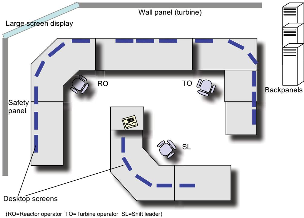
Figure 3. The layout of the case study nuclear control room (all measures not exactly to scale).
