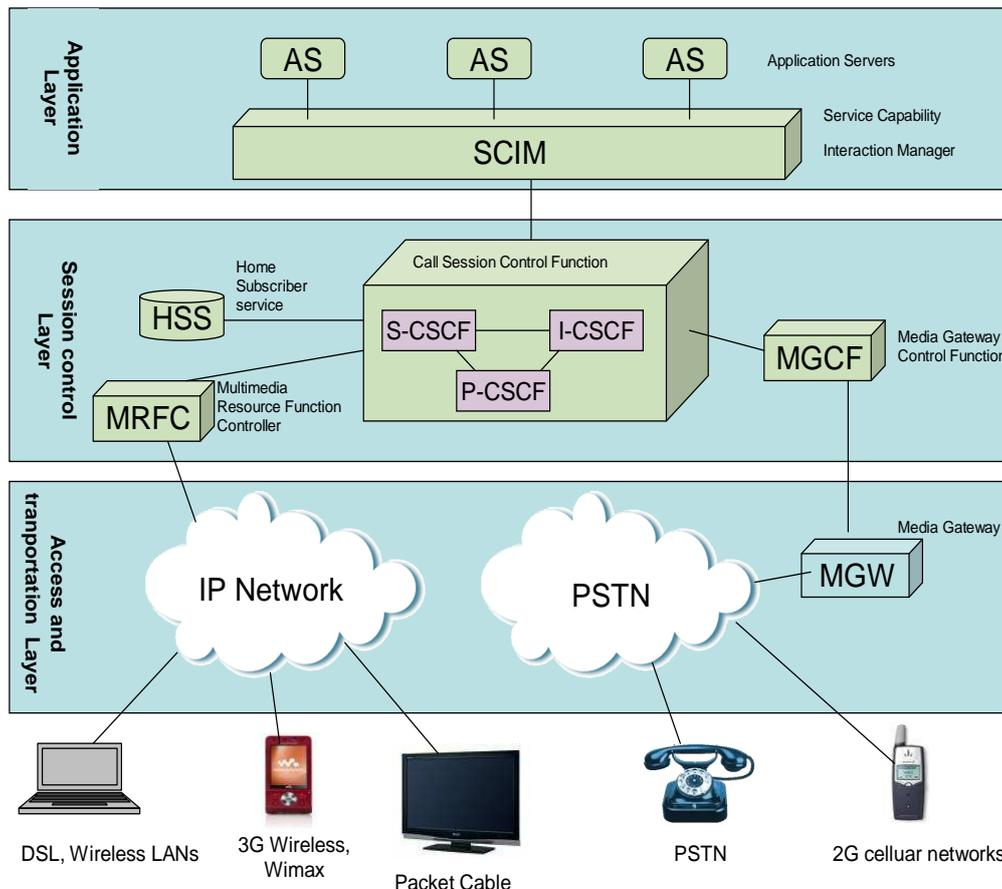
Figure 3- The IMS architecture has three layers. The Applications layer has the applications that can be used with IMS, the Session control layer is the brain of the architecture and the Access and Transport layer has the possibility to connect different networks to IMS.
