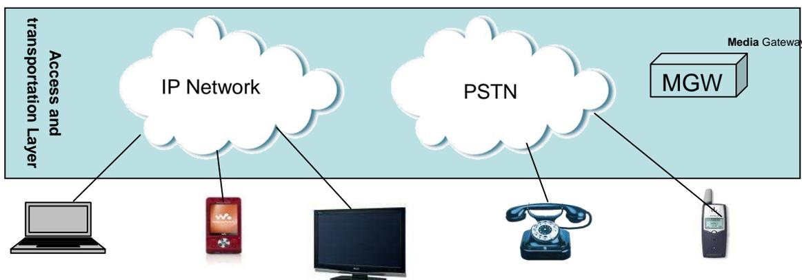
Figure 4 - To access and transport layer can different devices be connected such as mobile phone, fixed telephony, TV and computer. The description under each device shows which network is used to connect to the access and transport layer.
