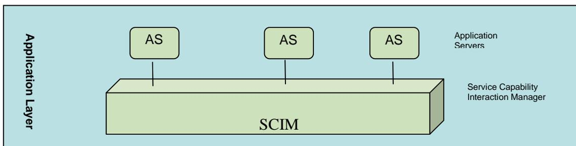
Figure 5 - The application layer has two key components; the application server and the service capability interaction manager. New applications are added to the application server while the SCIM keep in track which devices that works with different applications.
