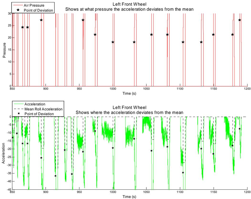
Figure 19. The top graph shows at what pressure the acceleration deviates from the mean, marked with black stars. The bottom graph shows the pre-braking mean acceleration, dashed black line, the acceleration data, solid green line, and the points of deviation from the pre-braking mean, marked with a black star. The deviation is calculated using the unmodified WECO-rules.
