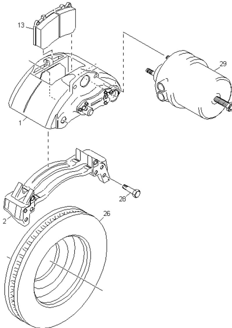
Figure 6. The figure shows some of the components in the air disc brake in the electronic brake system. The brake disc (26) and the brake pads (13), in this figure only one brake pad, make up the friction pair. The brake chamber(29)and the brake calliper (1) make up the other parts of the air disc brake.
