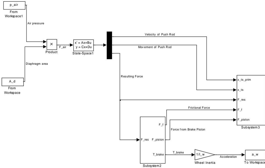
Figure 16. The figure shows the Simulink model that was used in the model based method for extracting the application pressure.
