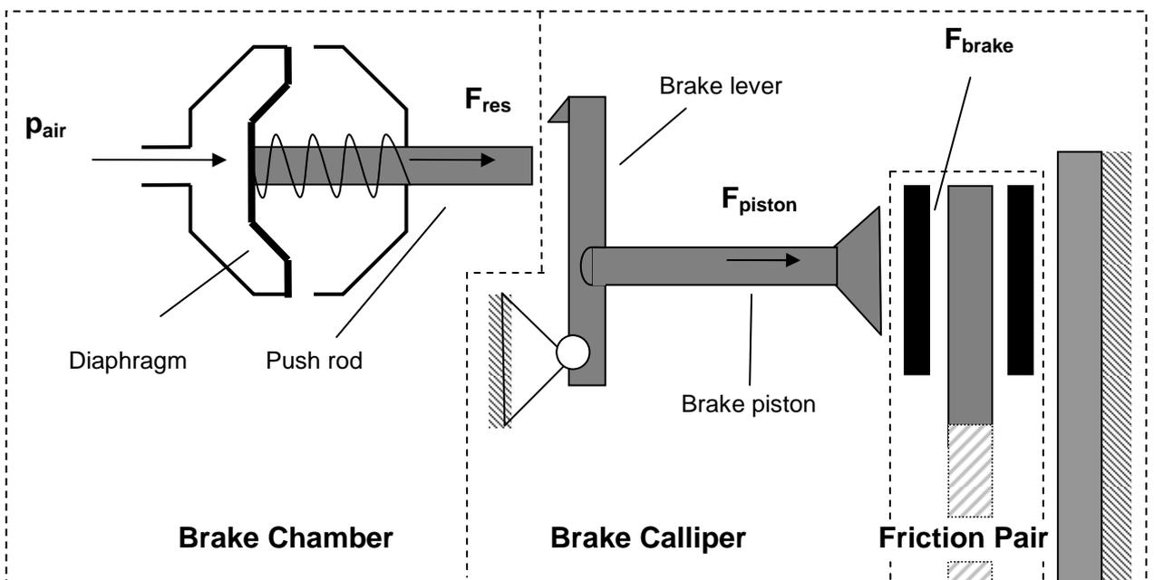
Figure 4. Schematic picture of the Air Disc Brake. The dashed lines mark the boundaries for the different parts of the system; Brake Chamber, Brake Calliper and Friction Pair (Based on Harju, 2008-01-28).
