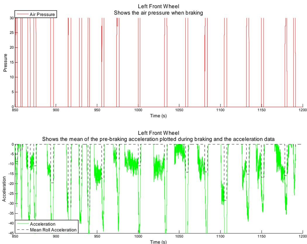
Figure 18. The top graph shows the air pressure when braking and the bottom graph shows the mean pre-braking acceleration, dashed black line, and the acceleration data, solid green line. The mean pre-braking acceleration is calculated during the pre-braking, but plotted during braking to make the comparison with the acceleration data easier.
