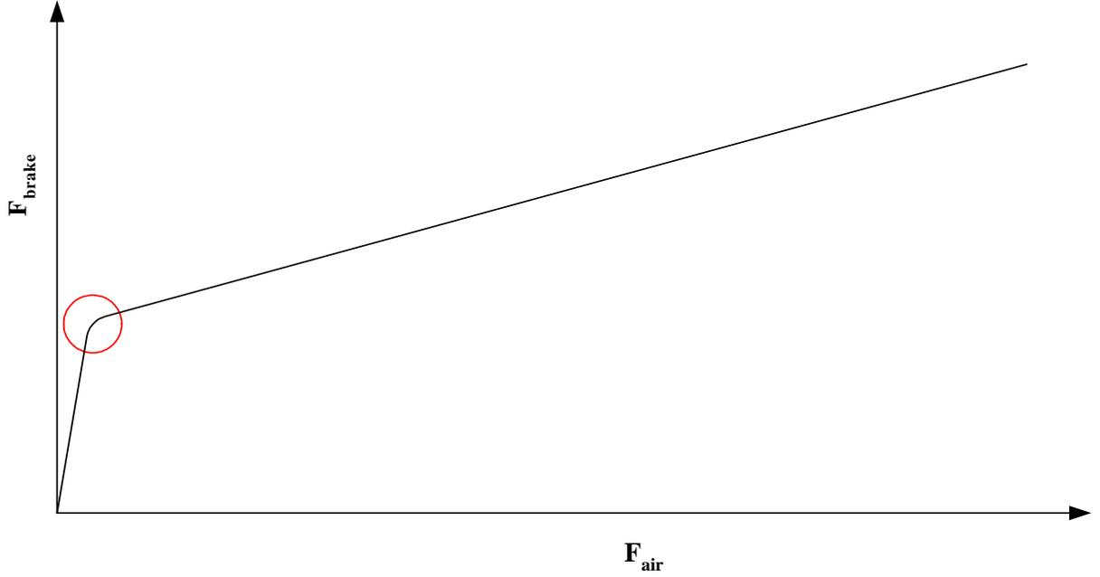
Figure 14. The graph shows how the force applied on the brakes,  $F_{brake}$ , changes when the brakes have applied, which the red circle indicates. Since the acceleration of the wheel depends on the brake force this means that the acceleration has the same nonlinear properties as the brake force (Based on Harju & Löfstrand, 2007-10-10).
