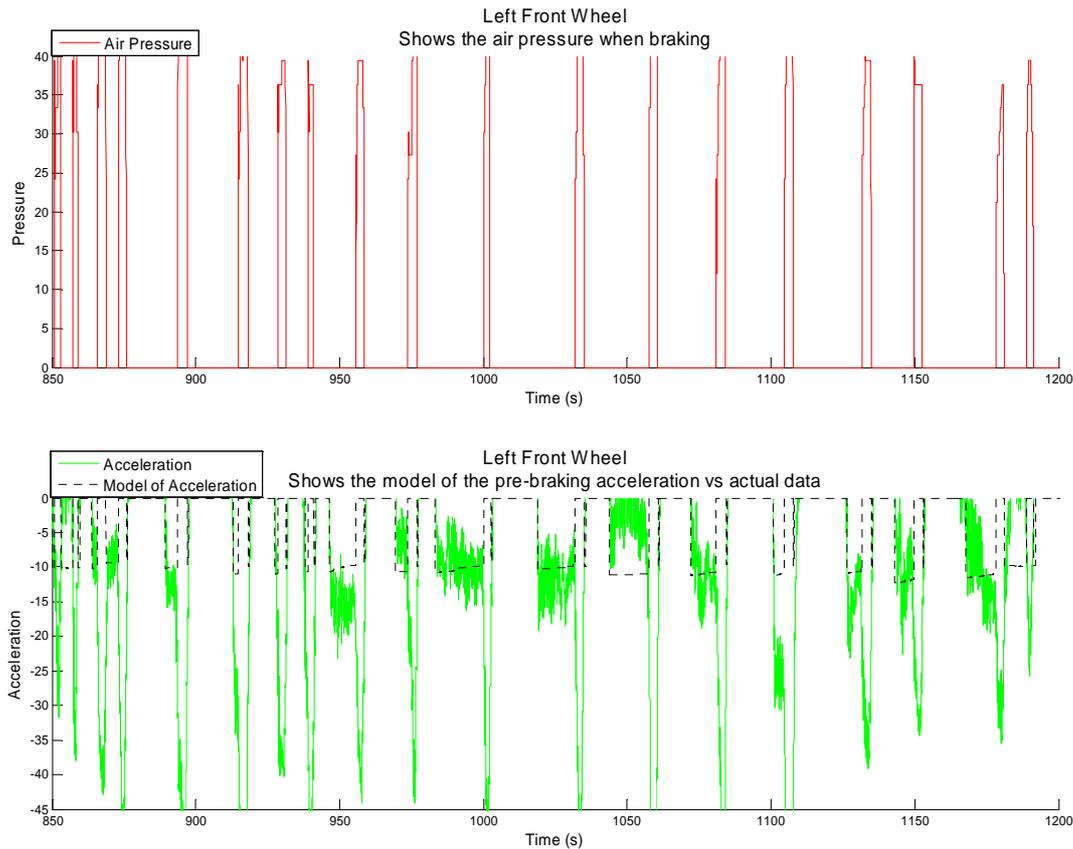
Figure 17. The top graph shows the air pressure when braking and the bottom shows the model of the rolling, pre-braking acceleration, dashed black line, compared with the acceleration data, solid green line. The model only emulates the sequence prior to braking.
