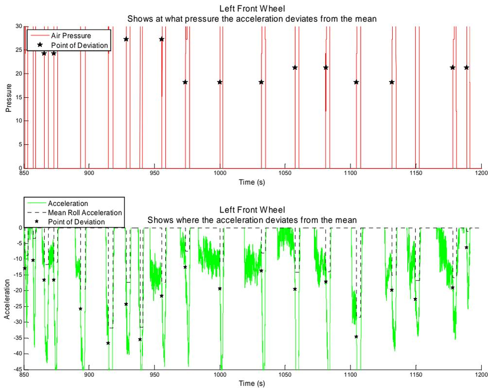
Figure 20. The top graph shows at what pressure the acceleration deviates from the mean, marked with black stars. The bottom graph shows the pre-braking mean acceleration, dashed black line, the acceleration data, solid green line, and the points of deviation from the pre-braking mean, marked with a black star. The deviation is calculated using the modified WECO-rules.
