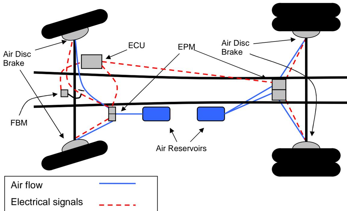
*Figure 3. Schematic overview of the Electronic Brake System (EBS) in a truck. The red dotted lines show how the electrical signals are transmitted between the components and the blue lines show how the air flows from the reservoirs and is controlled from the EPMs.*
