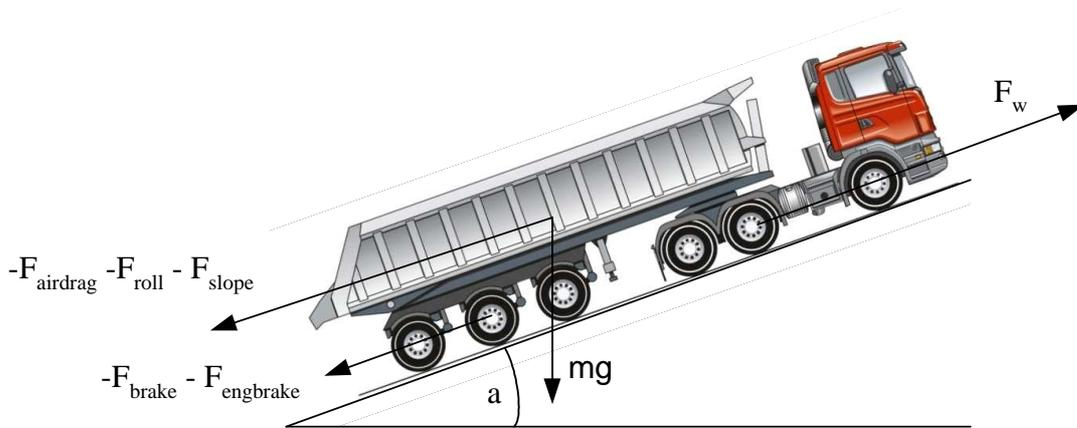
Figure 8. The figure illustrates the forces that affect the truck (Based on Eriksson & Nielsen, 1998, p 112).
