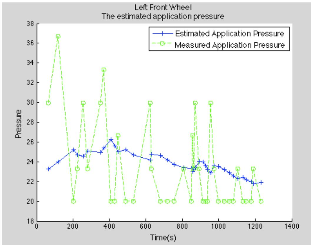
Figure 21. The graph shows the estimated application pressure in relation to the measured application pressure.
