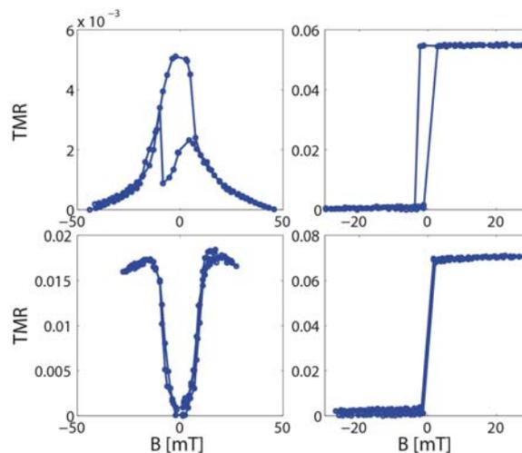
**Fig. 5.** TMR measurements of the MTJs from the FIB process (top row), and from the ESCA process (bottom row). The magnetic field was applied both along the hard axis (left column) and the easy axis (right column).
