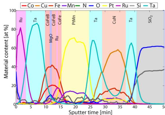
**Fig. 3.** Depth profile for etching in ESCA..
