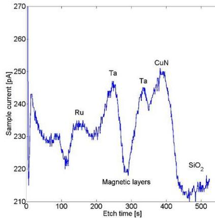
**Fig. 1.** End point detection profile of the TMR used as reference in the MTJ patterning process using FIB.
