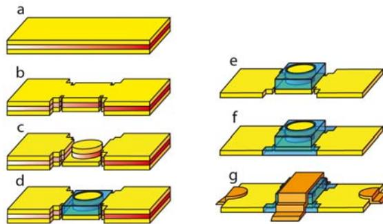
**Fig. 2.** Scheme of the FIB-based MTJ manufacturing process.
