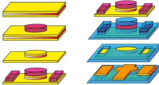
**Fig. 4.** Scheme of the MTJ fabrication process using ESCA equipment.
