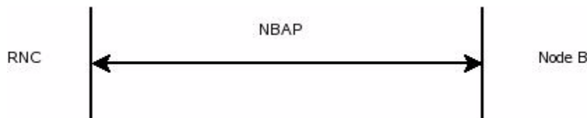
Figure 2-3. RNC and Node B signalling via NBAP
