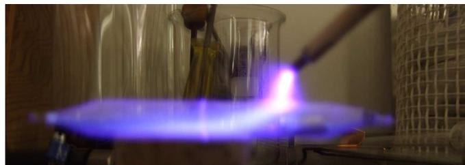
**Figure 3.1:** Spark tester induces plasma in the evacuated quartz tube.
