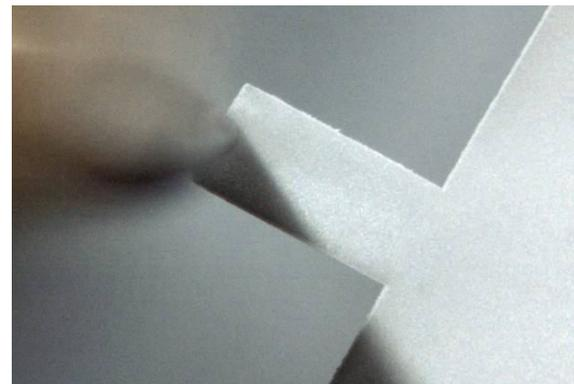
*Figure 3: Optical microscope image of an 800 μm long, 400 μm wide and 12 μm thick cantilever beam. Dimensions after firing. A pin is placed at the tip of the beam.*
