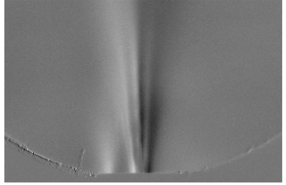
Figure 7: Exhaust from thruster chip #1 in vacuum, cut-off parallel to exhaust jet. The lighter area to the left of the jet is due to leaking gas. Field of view is  $7 \times 4.5$  mm.
