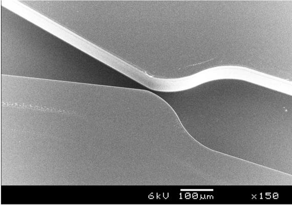
Figure 1: Image of a micronozzle manufactured using DRIE. Gas is exhausted to the left.
