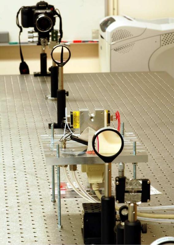
Figure 3: Final setup. From bottom right to top left: variable slit, collimating lens, test area, schlieren lens, cut-off, and camera with mounted lens and bellows.
