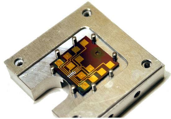
Figure 4: Thruster chip (22×22 mm) in opened fixture. The U-shaped spacer and eight alignment pins surround the silicon chip. The thruster exhausts into the milled groove in the bottom left of the picture. Here, 12 connector pads are used to drive the heaters.
