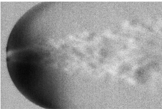
Figure 6: Exhaust from thruster chip #1 photographed with cut-off perpendicular to flow,  $1/1000$  s exposure time, ISO 1600. Notice the darker area close to the nozzle due to leakage. Field of view is  $21 \times 14$  mm.
