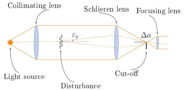
Figure 2: Simplified schlieren set-up, with  $\varepsilon_y$  denoting angle of refraction of a light ray, and  $\Delta a$  the resulting displacement at the cut-off.
