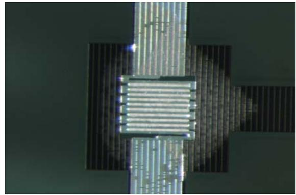
Fig.3. Microscope image of a FMMR chip. The expansion slots, 10  $\mu\text{m}$  wide and 220  $\mu\text{m}$  long, are visible as light rectangles between the heater meander. The light area in the oxide is light going through the thick oxide membrane.
