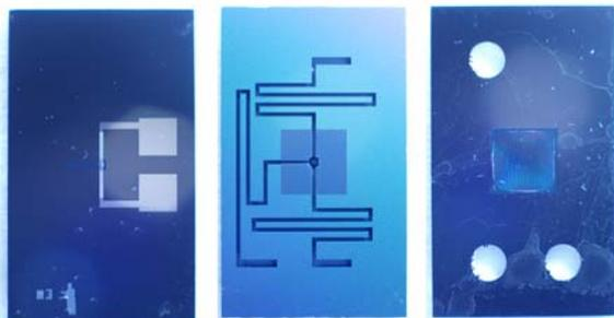
Fig. 2. Overview images of the top chip frontside (left), its backside (middle), and bottom chip frontside (right).
