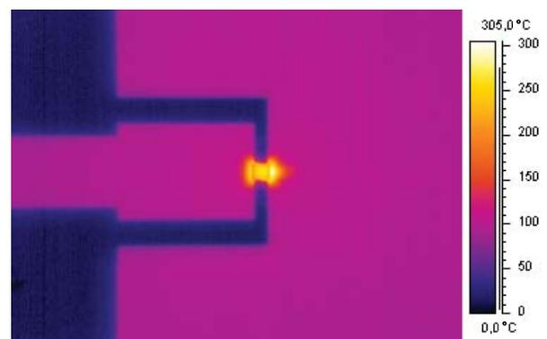
Fig. 5. Infrared image showing the difference in temperature distribution when device I is heated with 1 W and with the heater switched off.
