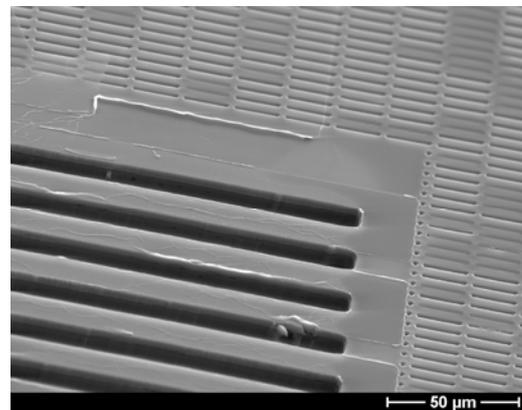
Fig.4. SEM image of the FMMR expansion slots (large openings), surrounded by the aluminium heater and silicon via which is embedded in the thick oxide where the pattern after the etched trenches is still visible.
