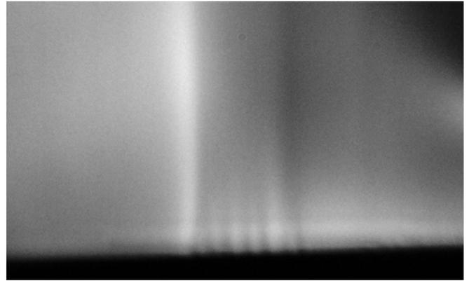
Fig.7. Schlieren image of exhausted gas from a FMMR chip with seven different thruster units expelling pressurized xenon. The distance between the jets furthers to the right and left is about 600  $\mu\text{m}$ .
