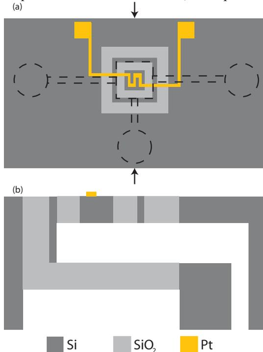
Fig. 1. Schematic of the microreactors with: (a) top view, and (b), cross section along the line indicated by arrows in (a).
