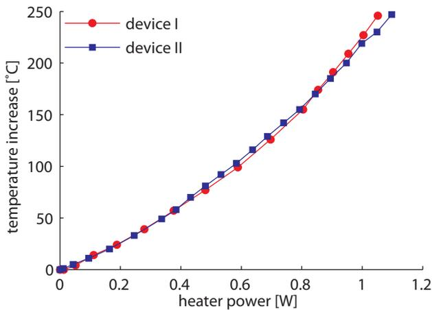
Fig. 6. The temperature increase of the silicon via on top of the chamber for different supplied power level. The temperature is here measured with an infrared camera.
