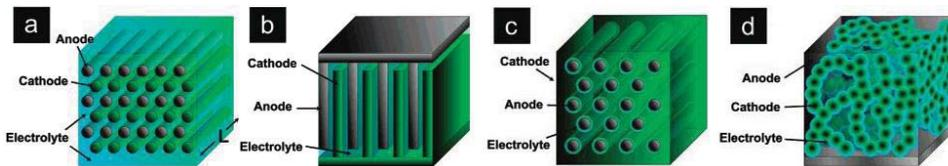
Figure 2: Geometrical structures of 3-D battery cells [6]
