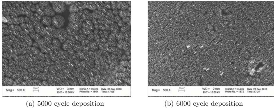
Figure 3: Nanorod deposition at different cycles with a pulsed current of -5 mA (0.2 s)/0 A (2 s)
