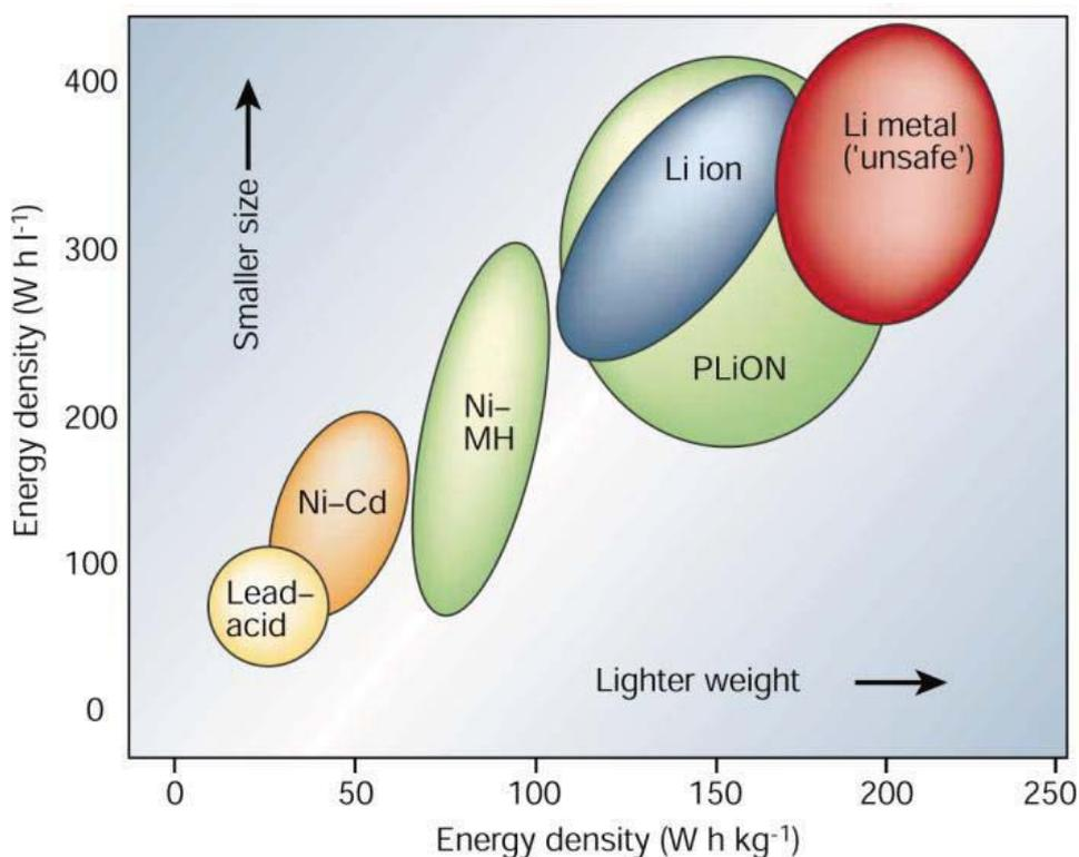
Figure 1: Comparison of energy density for different battery systems [1]
