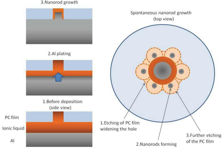
Figure 7: Aluminium nanorod growth mechanism
