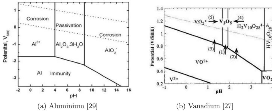
Figure 8: Pourbaix diagram for vanadium and aluminium species in an aqueous solution
