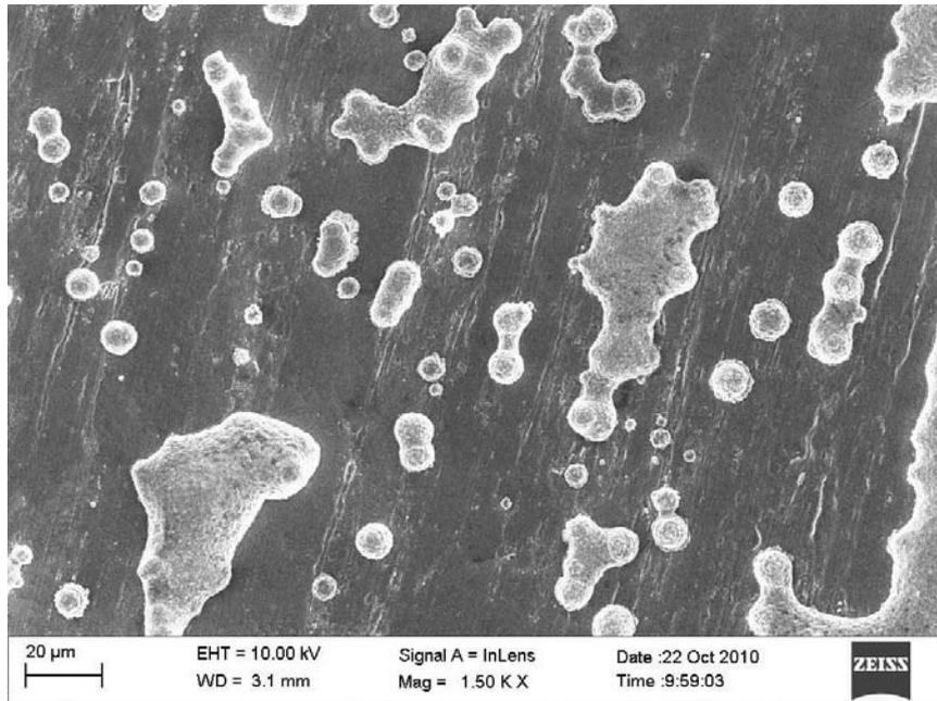
Figure 5: Nucleations in the deposition with a PC film without pores, deposited with a pulsed current of  $-5 \text{ mA}$  ( $0.2 \text{ s}$ )/ $0 \text{ A}$  ( $2 \text{ s}$ )
