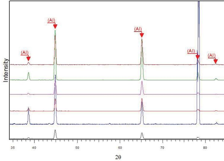
Figure 9: XRD analysis of the pH dependence of vanadium oxide deposition. From bottom and up; aluminium reference sample(black), pH 2(blue), pH 2.5(red), pH 3(purple), pH 3.5(green), pH 4(dark red). The red peaks correspond to aluminium (cubic).
