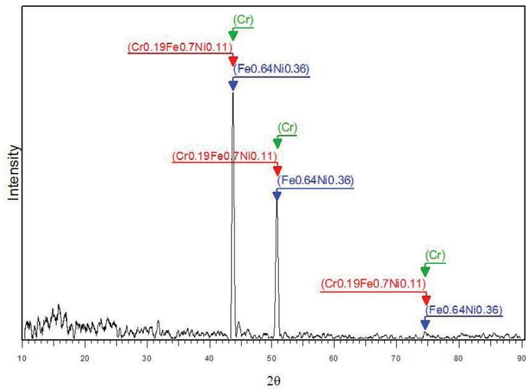
Figure 10: XRD analysis of vanadium oxide deposition on a stainless steel sample. Possible phases are: Iron Nickel ( $Fe_{0.64}Ni_{0.36}$ )(blue), Chromium Iron Nickel ( $Cr_{0.19}Fe_{0.7}Ni_{0.11}$ )(red), Chromium (Cr)(green).
