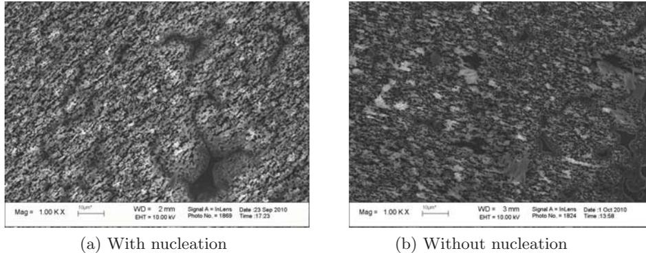
Figure 4: Comparison of deposition with and without nucleation pulse, deposited with a pulsed current of  $-5 \text{ mA}$  ( $0.2 \text{ s}$ )/ $0 \text{ A}$  ( $2 \text{ s}$ )
