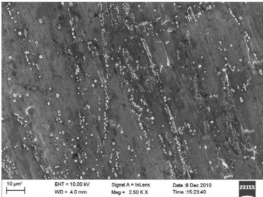
Figure 6: Homogeneous nucleation on aluminium sample in the PC film with pores experiment, deposited with a pulsed current of  $-5 \text{ mA}$  ( $0.2 \text{ s}$ )/ $0 \text{ A}$  ( $2 \text{ s}$ )
