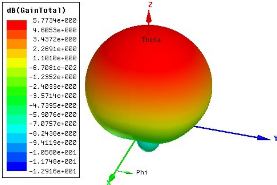
Figure 3.7: The simulated gain of the second patch antenna
