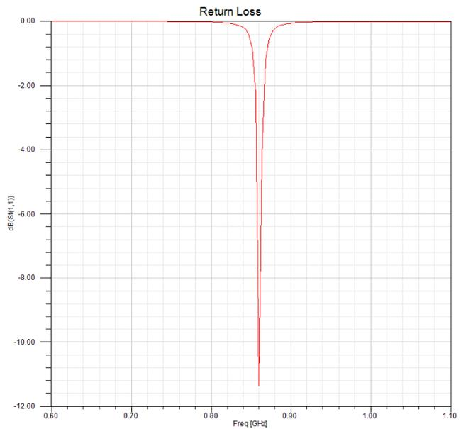
Figure 3.8: The simulated input impedance of the second patch antenna
