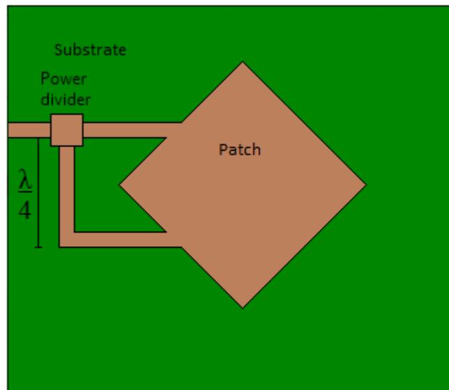
Figure 2.14: Patch antenna with circular polarization by dividing the signal
