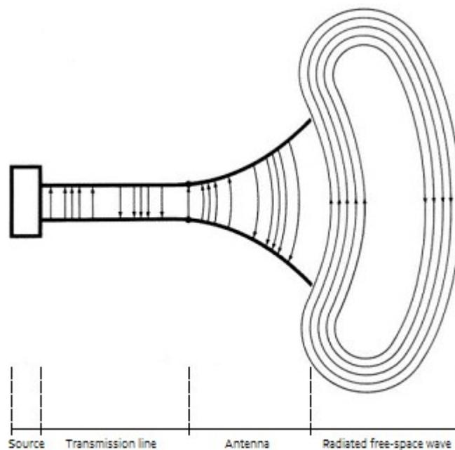
*Figure 2.1: The concept of a basic antenna setup*
