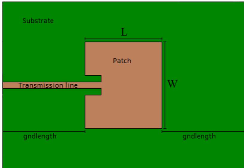
Figure 3.10: A patch antenna showing how the variable gndlength affected the simulations of the antenna
