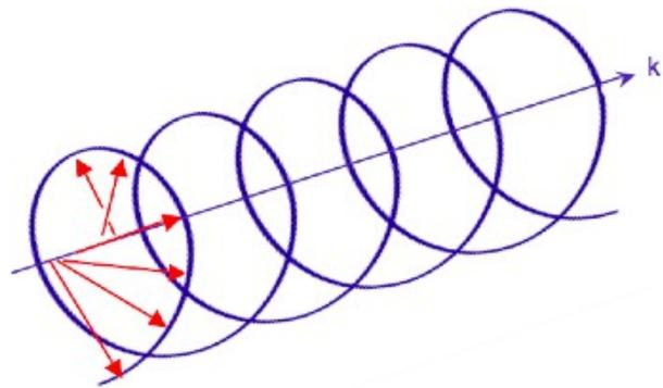
Figure 2.13: Circularly polarized waves
