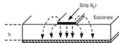
Figure 2.6: Field lines for a microstrip transmission line
