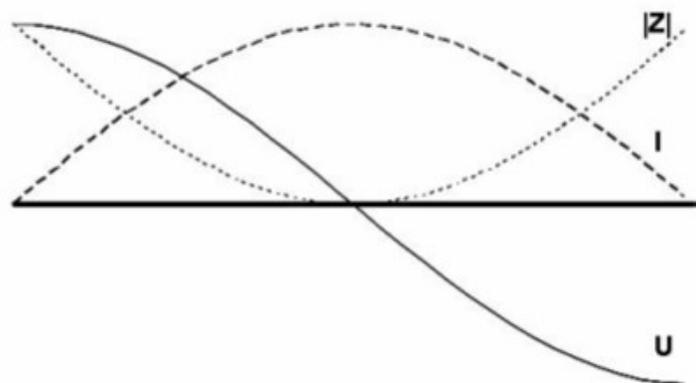
Figure 2.8: The impedance ( $|Z|$ ), current ( $I$ ) and voltage ( $U$ ) distribution for the patch in a patch antenna
