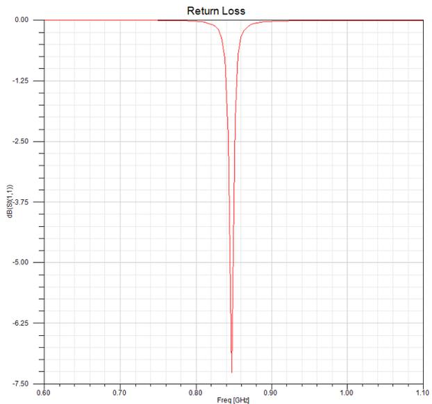
Figure 3.5: The simulated return loss of the first patch antenna
