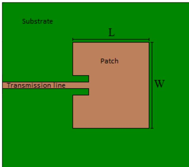
Figure 2.9: Inset-fed patch antenna
