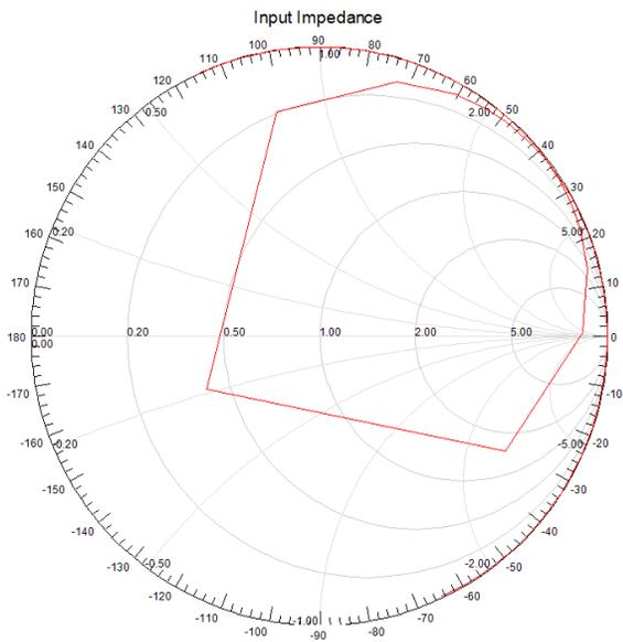
Figure 3.4: The simulated input impedance of the first patch antenna
