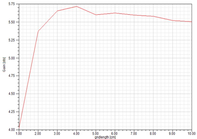
Figure 3.11: The simulation for comparing different sizes of the ground plane length
