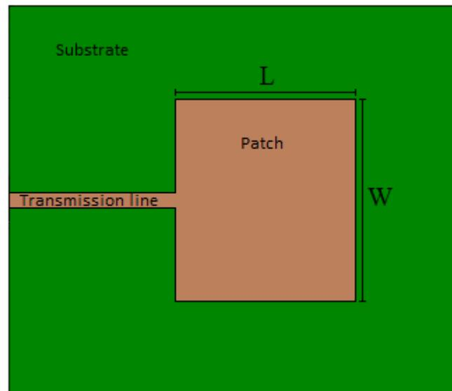
Figure 2.4: A basic patch antenna with length  $L$  and width  $W$  and a microstrip transmission line
