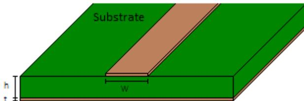
Figure 2.5: A side view of a microstrip transmission line
