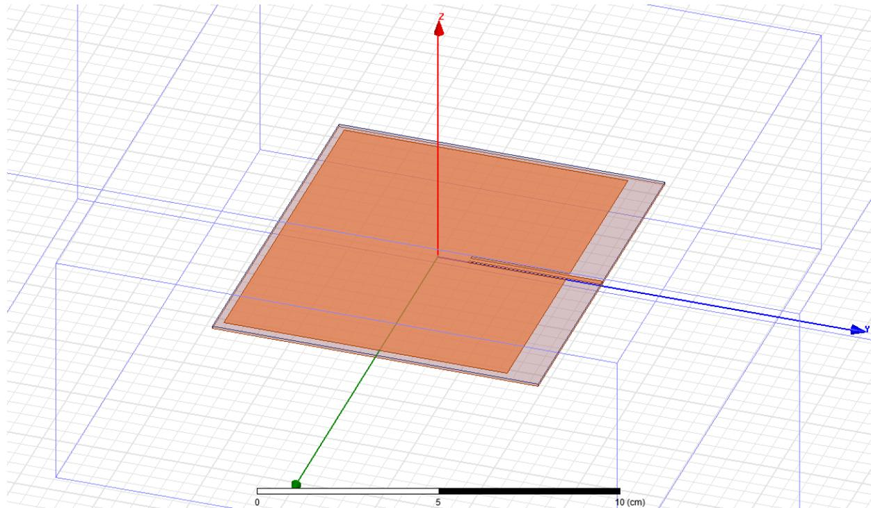
*Figure 3.2: The first patch antenna created in HFSS*
