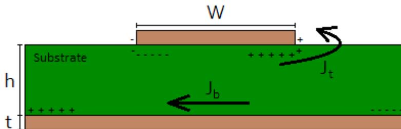
Figure 2.7: Current distribution for a patch antenna
