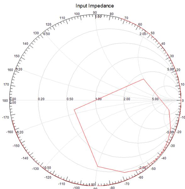
Figure 3.9: The simulated input impedance of the second patch antenna
