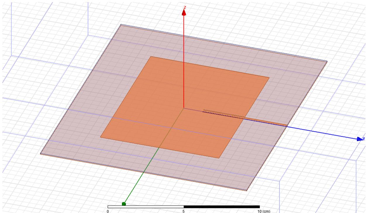
Figure 3.6: The second patch antenna created in HFSS
