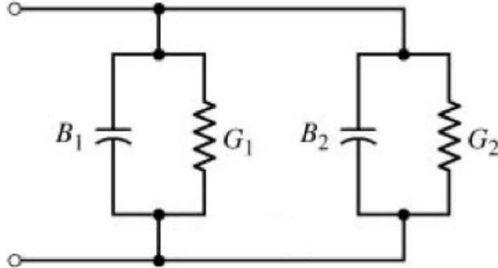
Figure 2.11: Equivalent circuit of the two radiating slots
