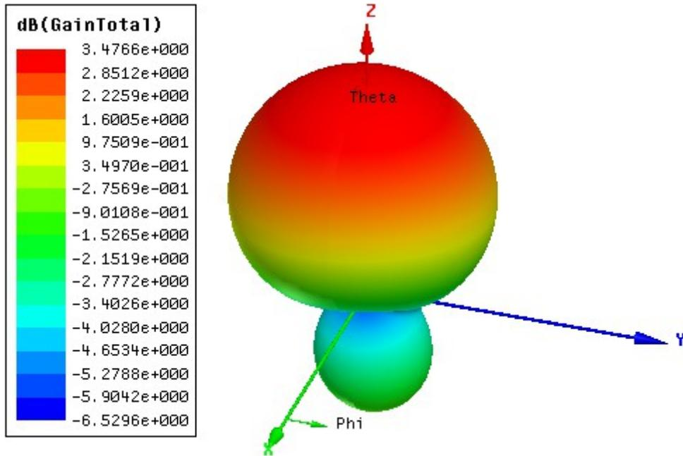
Figure 3.3: The simulated gain of the first patch antenna
