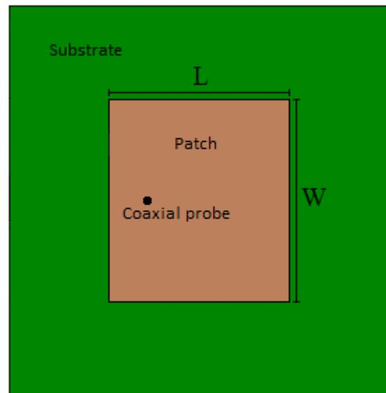
Figure 2.10: Probe-fed patch antenna
