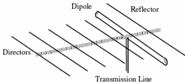
Figure 2.3: A Yagi-Uda antenna
