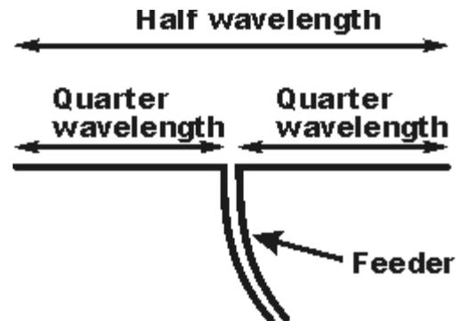
Figure 2.2: A dipole antenna
