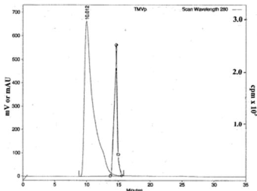
Fig 3. HPLC-separation on SUPELCO SigmaCrom GFC-100 protein Column; buffer: 0.1mM  $\text{NH}_4\text{HCO}_3$ , pH7.8; Continuous line: UV-absorbance at 280 nm; - o - : replicase activity expressed as cpm
