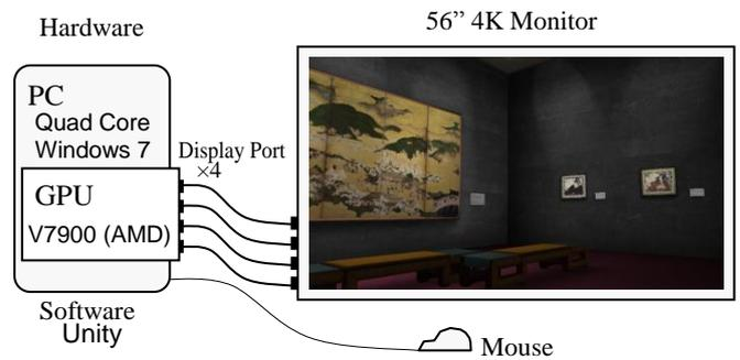
Figure 2. System configuration
