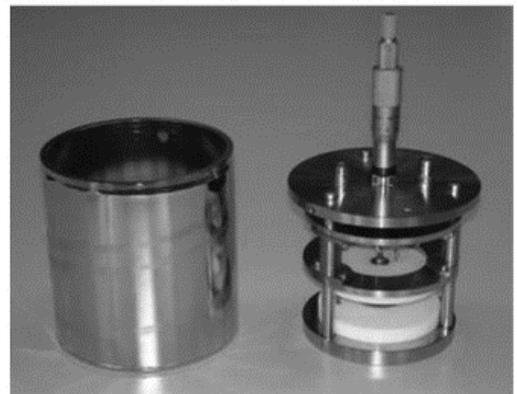
Figure 3.3 Image showing the Novocontrol Alpha-AN dielectric sample holder. Reprinted with permission.
