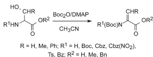
Scheme 7 Synthesis of protected dehydroamino acids using Boc<sub>2</sub>O/DMAP.<sup>40</sup>
