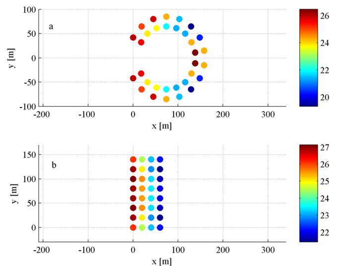
FIG. 2. Global geometry of the double circle segment array in (a) and the rectangular array in (b). Each dot corresponds to a WEC and the colors correspond to respective WECs CWR with the magnitude in percent given by the color bar. The sea state in this case has an energy period of 5.19 s and a significant wave height of 1.07 m. The wave is moving in the positive x-direction.
