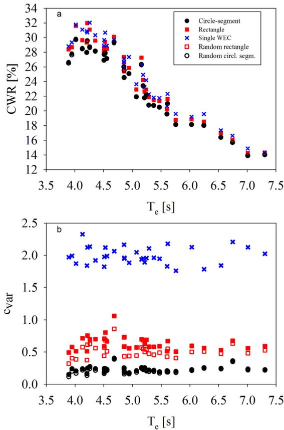
FIG. 4. Average CWR as a function of  $T_e$  in (a) and  $c_{var}$  as a function of  $T_e$  in (b). Black dots correspond to the circle-segment array with 32 WECs, red squares to the rectangular array with 32 WECs, and blue dots represent a single isolated WEC. Non-filled dots and squares correspond to rectangular and circle-segment arrays with randomized WECs. The average is taken over the 32 WECs.
