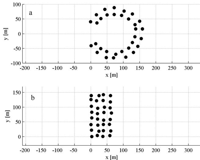
FIG. 3. Randomized circle segment array in (a) and randomized rectangular array in (b).
