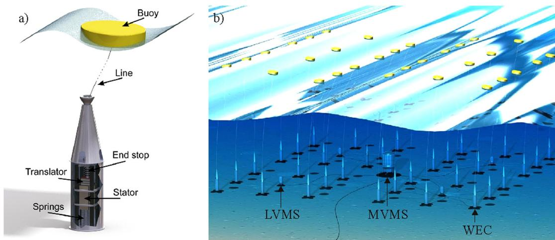
FIG. 1. The Uppsala University WEC in (a). A conceptual sketch of a future commercial scale wave power farm in (b).
