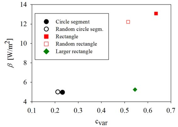
FIG. 5. Average power production density versus average normalized variance. The average is taken over the 34 sea states in Table I.
