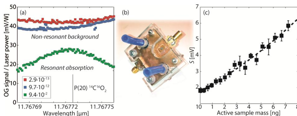
**Figure 1.** (a) Scaled optogalvanic signal as a function of wavelength around the P20 line of  $^{14}\text{C}^{16}\text{O}_2$  at  $^{14}\text{C}$  concentrations between  $2.9 \times 10^{-13}$  and  $9.4 \times 10^{-2}$  and pressures between 40 and 470 Pa. (b) Photograph of a stripline split-ring resonator plasma source. (c) Optogalvanic signal as a function of the active sample mass, i.e., the mass of carbon in the plasma cell of the stripline split-ring resonator.
