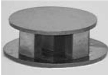
Figure 2: Piezoelectric proportional valve (14x5 mm) with microfabricated silicon parts
