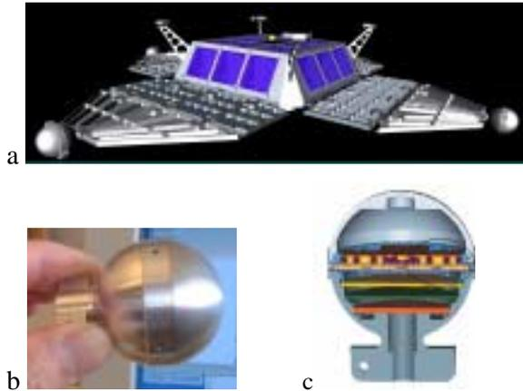
Figure 1: a) The nanosatellite under development at Angstrom Space Technology Centre, Uppsala University, Sweden. b) and c) The 60-grams autonomous thruster unit with four nozzles, designed for thrust level 0-10 mN.
