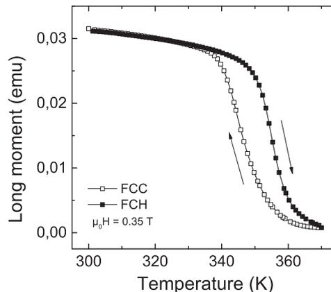
**Fig. 4.** Magnetization vs. temperature data of  $(\text{Fe}_{0.45}\text{Mn}_{0.55})_2\text{P}_{0.50}\text{Si}_{0.50}$ .
