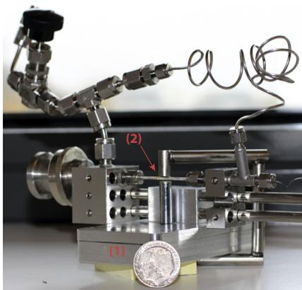
**Fig. 1.** Sample cell for SR-XRPD experiments in a magnetic field. A permanent magnet of NdFeB-type is placed inside the aluminum box (1). Samples placed in the gap (2) are exposed for a magnetic field of 0.35 T.
