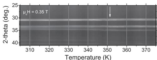
**Fig. 2.** Diffraction intensities vs. temperature for  $(\text{Fe}_{0.45}\text{Mn}_{0.55})_2\text{P}_{0.50}\text{Si}_{0.50}$ . Collected in a magnetic field of 0.35 T.
