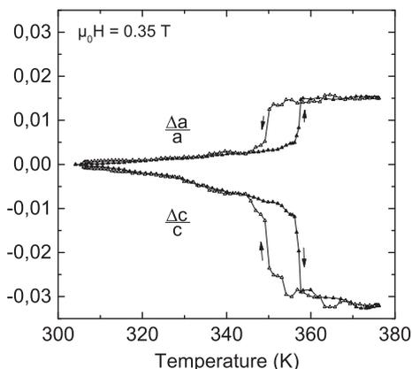
**Fig. 3.** The relative changes of the unit cell parameters of  $(\text{Fe}_{0.45}\text{Mn}_{0.55})_2\text{P}_{0.50}\text{Si}_{0.50}$  vs. temperature. Data were collected in a magnetic field of 0.35 T.
