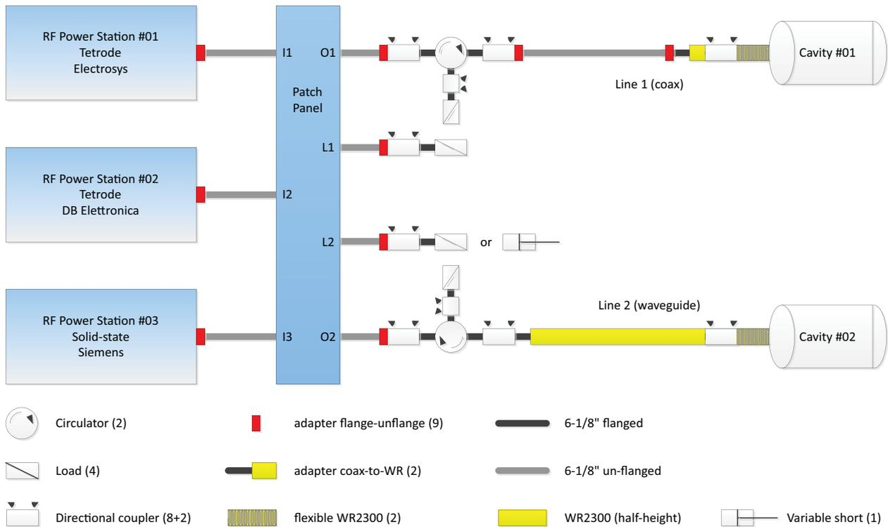
Figure 6: Test configuration for the cryomodule.
