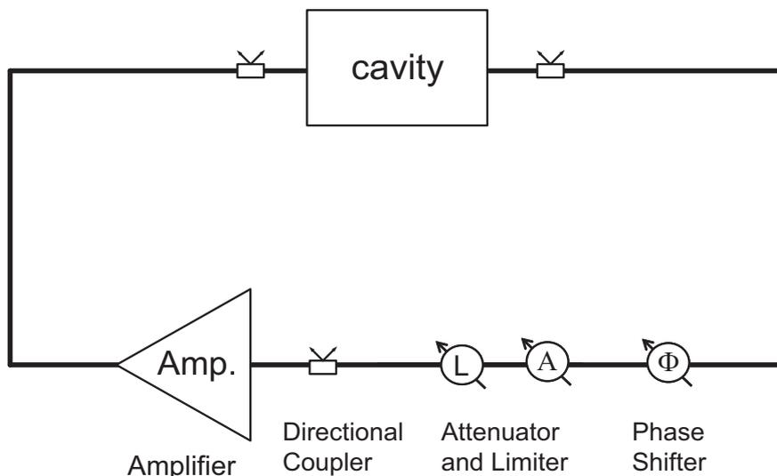
Figure 4: Test configuration of a bare cavity with self-excited loop.
