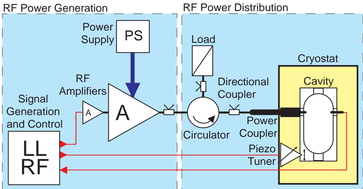
Figure 5: Test configuration of a high power RF amplifier and spoke cavity.
