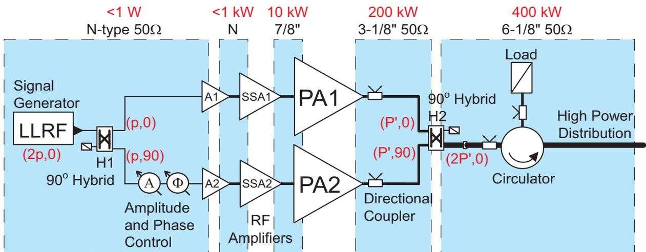
Figure 3: Layout of the high power RF amplifier. A1, A2 are solid-state drivers, SSA1 and SSA2 solid-state pre-amplifiers and PA1, PA2 tetrode power amplifiers.
