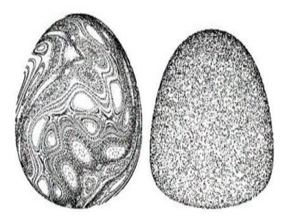
Poincaré sections of a passive tracer which visualize two different patterns; left: combination of many islands embedded in chaotic areas, right: a chaotic sea. Taken from [3]
