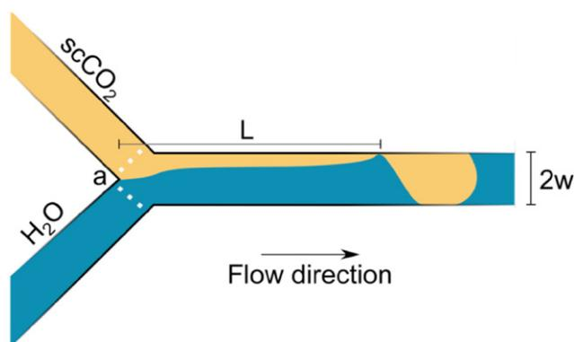
**Figure 1.** The inlets of the channel with the width  $2w$ , where  $Re$ ,  $Ca$ , and  $We$  are calculated for  $\text{H}_2\text{O}$  and  $\text{CO}_2$  at the position  $a$ , marked by dotted lines. The parallel length  $L$  is measured as the distance from where the two flows meet to where the flow breaks up into segments.
