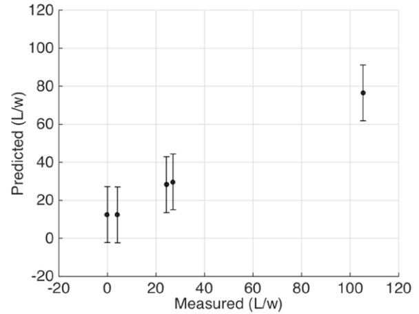
**Figure 8.** The measured parallel length compared to the predicted parallel length by the model for the parallel length. The error bars represent the RMSEP of the model of 14.6, i.e. and standard deviation of 1.4 mm.
