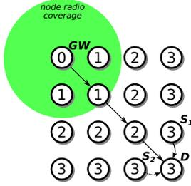
Fig. 4: Example of a 16-node grid network with uniform radio coverage. The numbers on nodes describe number of hops to gateway. *GW*: gateway node, *D*: destination node, *S<sub>1</sub>*: initial source node of a dataflow, *S<sub>2</sub>*: source node after task remapping. Straight arrows: task setup message path for node *D*; curved arrows: task-to-task dataflows.
