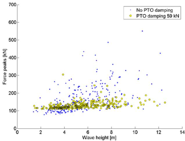
Fig 8. Measured force peaks in irregular wave tests  $I_1$  for the cylinder with moonpool float (CM), plotted against the individual wave height of the incident wave.
