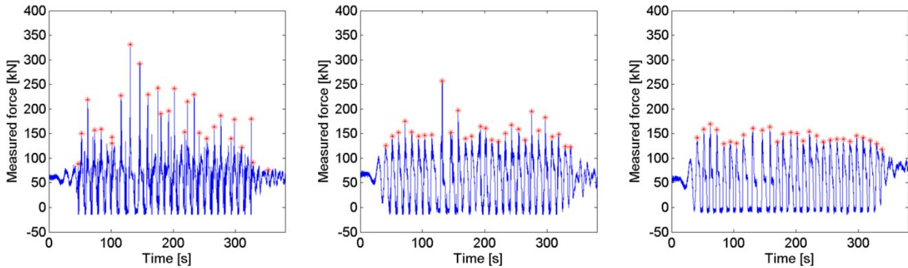
Fig 10. Force measurements for the embedded focused wave test T<sub>12</sub> with three different (approximate) values of the PTO damping: 18 kN (left), 59 kN (middle) and 83 kN (right).
