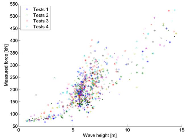
Fig 4. Force peaks in all 32 tests with focused waves embedded in regular wave backgrounds. In each tests, 22-28 force peaks have been identified and are plotted. The accumulation of data points in the wave height range 5-7 m correspond to the regular wave background.
