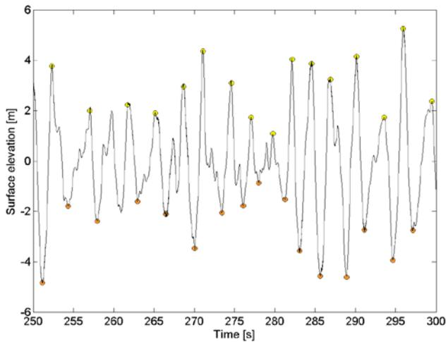
Fig 5. Surface elevation for the irregular wave test  $I_2$  as detected by a wave gauge in the direct vicinity of the cylinder (CYL) float.
