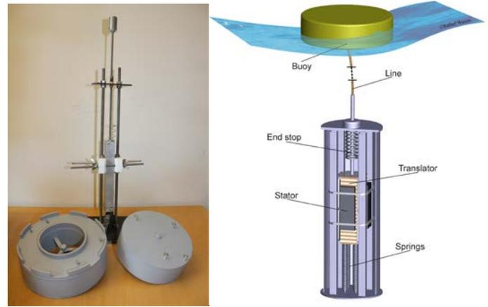
Fig 1. The model used in the experiments, and an illustration of the full-scale WEC. The full-scale PTO damping is electrical, whereas in the model it is asserted by friction brakes acting on the translator.
