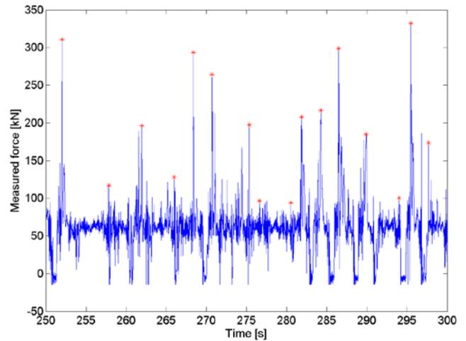
Fig 6. Force measurements for the irregular wave tests  $I_2$  for the cylinder float (CYL), as well as the identified force corresponding to each individual wave in Fig. 5.
