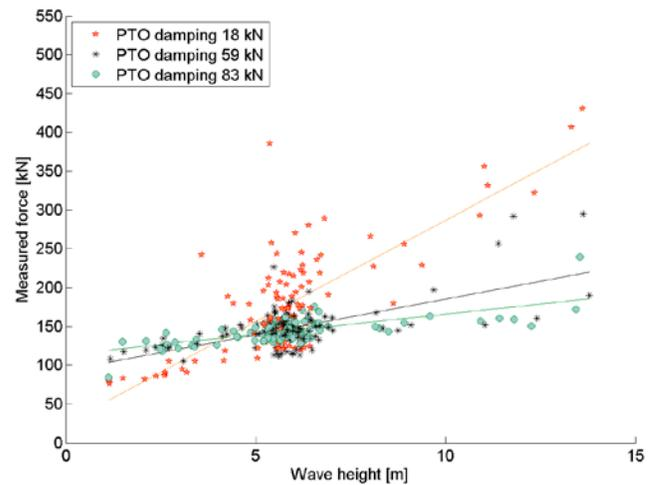
Fig 9. Measured force peaks in the embedded focused wave test T12 for the CWD float with the three different values of PTO damping. Linear trend lines have been added for visibility. Compare with Fig. 4 for the case without PTO damping.
