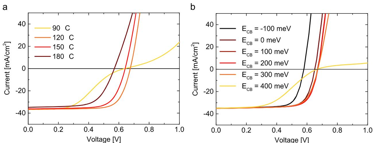
**Fig. 1.** (a)  $J$ - $V$  curves of the best solar cells, out of 12 cells on each sample, where the ZTO buffer layer is deposited with a Sn/(Sn+Zn) cycle fraction of 0.4 at deposition temperatures of 90 °C, 120 °C, 150 °C and 180 °C. (b) Simulated  $J$ - $V$  characteristics assuming different CIGS/ZTO conduction band offsets  $\Delta E_{CB}$ .
