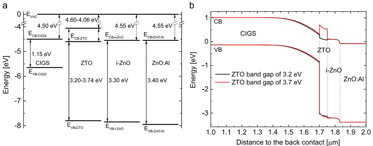
**Fig. 4.** (a) Schematic illustration of the band energy levels used in the SCAPS-1D simulations. (b) Zoomed in resulting band diagram for a simulated CIGS device with ZTO band gap of 3.2 eV and 3.7 eV at short circuit conditions.
