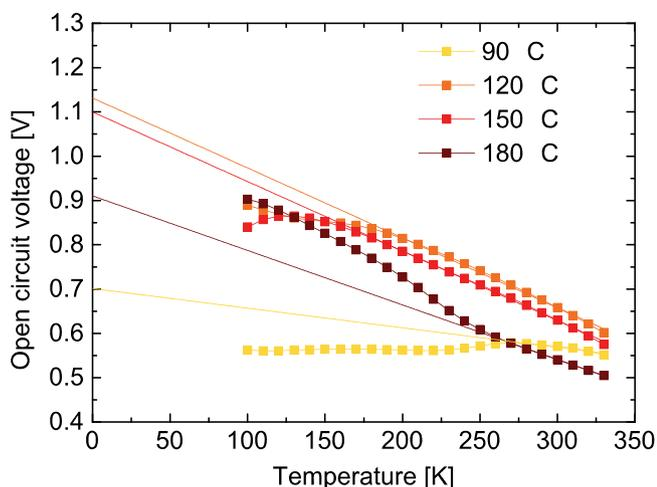
**Fig. 2.** Temperature dependence of  $V_{OC}$  of cells where the ZTO buffer layers are deposited with a Sn/(Sn+Zn) cycle fraction of 0.4 at deposition temperatures of 90 °C, 120 °C, 150 °C and 180 °C.
