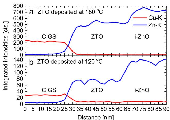
**Fig. 3.** EDS scans over the CIGS/ZTO interface, where the ZTO buffer layer is deposited by a Sn/(Sn+Zn) cycle fraction of 0.4. (a) The ZTO layer is deposited at 180 °C. (b) The ZTO layer is deposited at 120 °C.
