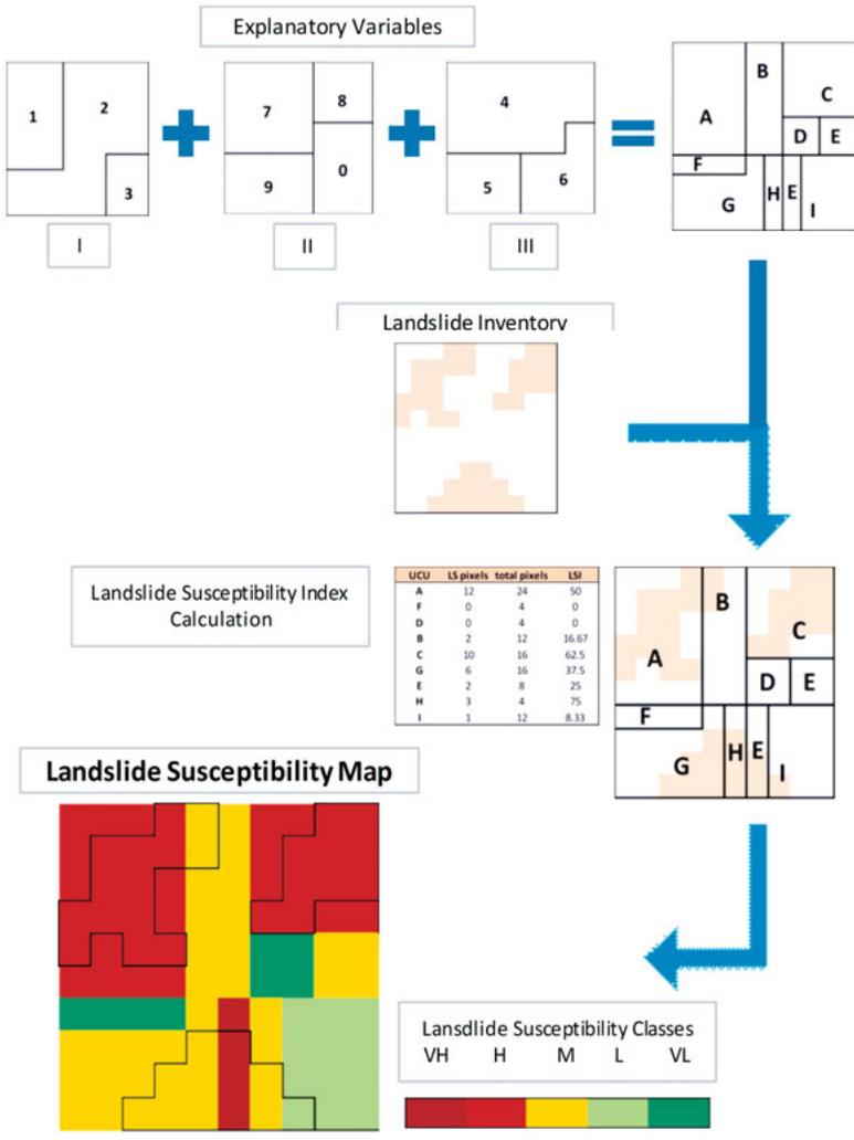
Figure 13. Methodology scheme for the construction of the susceptibility maps
