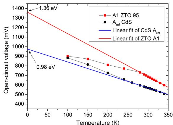
FIG. 4.  $V_{oc}(T)$  of  $A_{ref}$  (CdS) versus A1 (ZTO 95 °C). Within the linear region used for extrapolation, the ideality factor is confirmed to be temperature independent.
