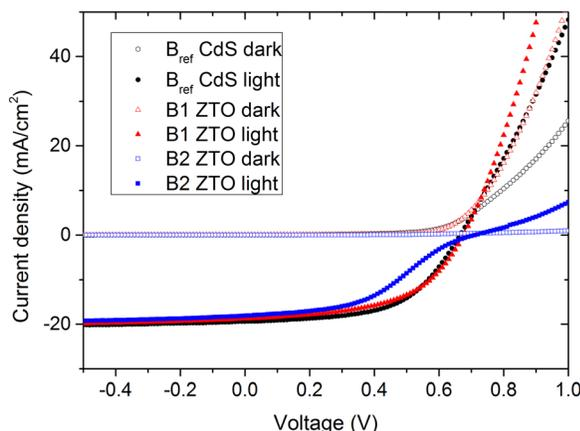
FIG. 3. IV curves of devices  $B_{ref}$ , B1, and B2; ZTO deposited at 120 °C and 80 °C.
