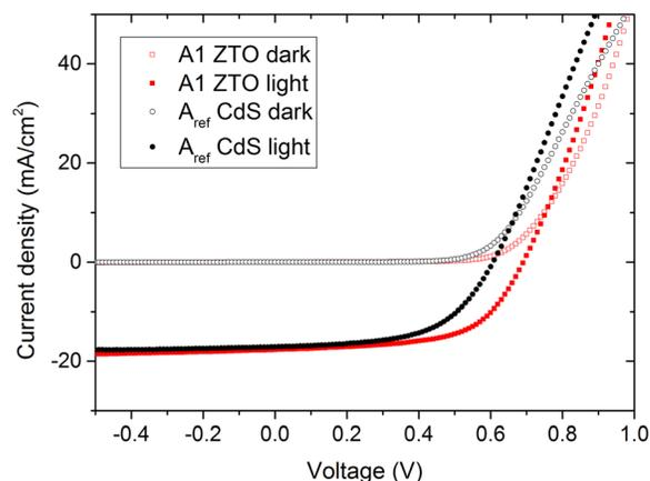
FIG. 1. IV curves of devices A<sub>ref</sub> and A1; ZTO deposited at 95 °C.
