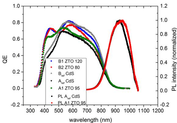
FIG. 2. EQE of all cells in Figs. 1 and 2 with normalized PL of devices  $A_{ref}$  and A1.
