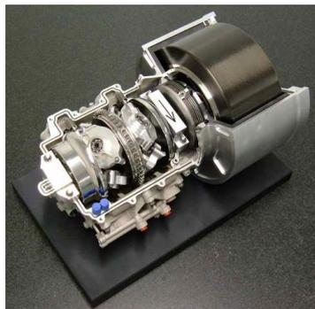
**Figure 3.** Flybrid Systems Formula 1 flywheel for the 2009 season. Note that the power requirements are quite high, and the mechanical power transfer system (a continuously-variable transmission) is a large part of the machine. Reprinted with permission from the copyright holder.
