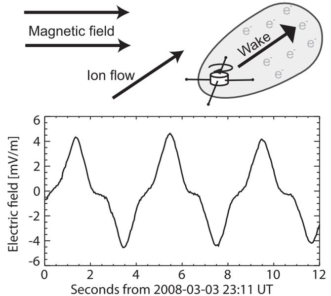
**Figure 3.** (top) Sketch of the wake behind a positively charged Cluster spacecraft, caused by a supersonic flow of cold ions. (bottom) Non-sinusoidal electric field measured by the electric field instrument booms on a Cluster spacecraft, in a supersonic flow of cold ions (André and Cully 2012, André *et al* 2015).
