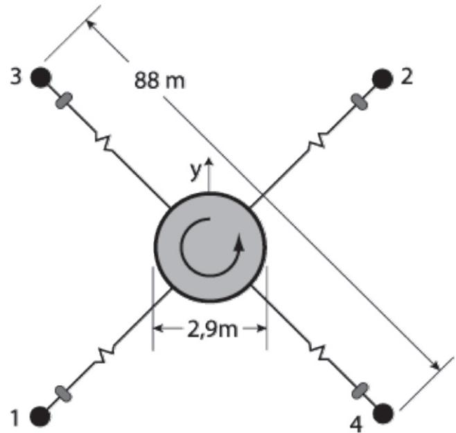
**Figure 2.** The electric field and wave (EFW) instrument has four wire booms mounted on each of the Cluster spacecraft. The distance from the satellite centre to the boom tip is 44 m. The satellite spins at a rate of once every four seconds, which keeps the booms taut. The actual sensor is a sphere, 8 cm in diameter, at the end of each boom.
