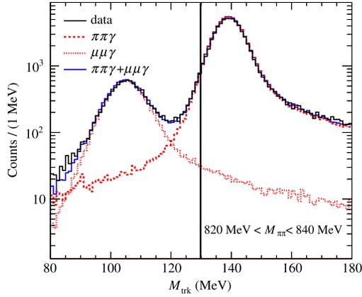
**Fig. 1.** Example of  $M_{\text{trk}}$  distributions for the  $M_{\pi\pi} = 820\text{--}840$  MeV bin. Measured data are represented in black, simulated  $\pi^+\pi^-\gamma$  and  $\mu^+\mu^-\gamma$  in red. Simulated  $\mu^+\mu^-\gamma + \pi^+\pi^-\gamma$  in blue. Events at the left of the vertical line are rejected. (For interpretation of the references to color in this figure legend, the reader is referred to the web version of this article.)
