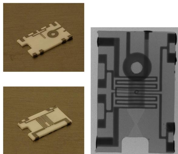
**Figure 3** Top and bottom of a completed microthruster (left), and an X-ray image (right) revealing the catalytic bed. The loops meeting at the centre of the heater are the temperature sensors on the top and bottom of the chip. The electrical connections over the edges are the darkest parts of the device, whereas the lightest part is the cavity with the inlet and nozzle.
