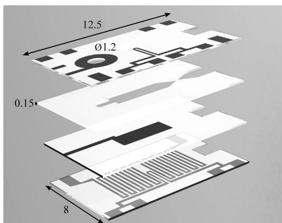
**Figure 1** Exploded view of thruster design. Bottom up: floor layer with heater and temperature sensor, catalytic layer, chamber wall layer with nozzle, and lid layer with propellant inlet, connection pads and temperature sensor (loop in the centre), on top. Note that the bottom layer is flipped over here. The heater is actually facing down. All dimensions are in mm and before sintering, where the component shrinks by approximately 20%.
