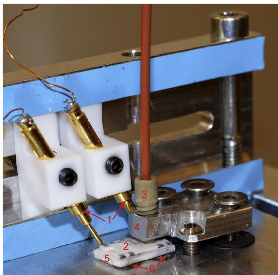
**Figure 2** Close-up of a chip partly mounted in the stainless steel fixture to show two (out of six) probes (1), the chip (2), the inlet connection (3), the steel cantilever beam clamp (4), the alumina piece below the chip (5), and the spring washers (6).
