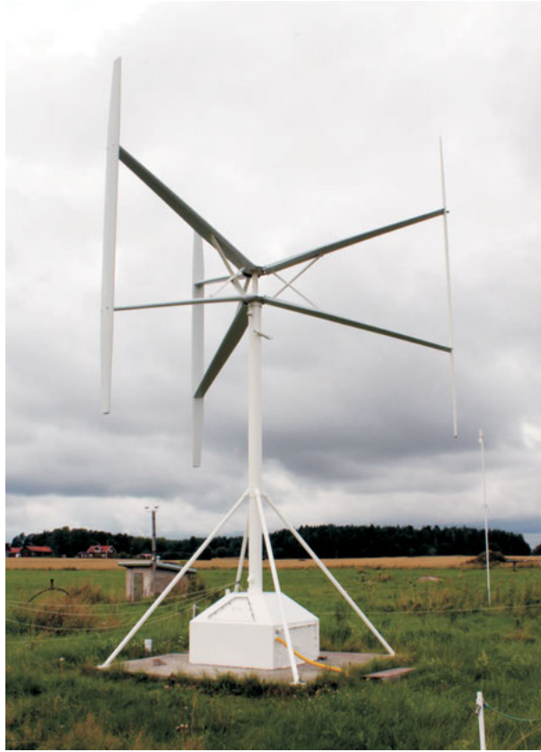
Figure 2.1. 12 kW vertical axis wind turbine designed and constructed at Uppsala University.
