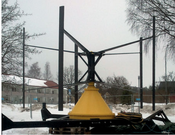
Figure 2.4. Prototype marine current energy converter before deployment in the river Dalälven, Sweden.
