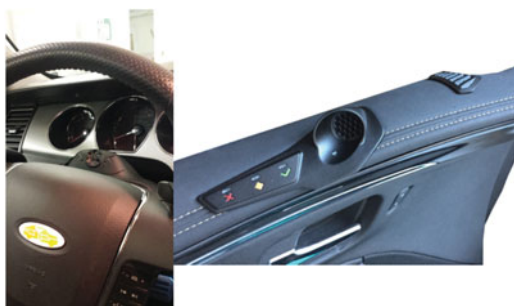
Figure 1. Sensors integrated into the casing of the steering column of a vehicle (left) and in the side door (right).
