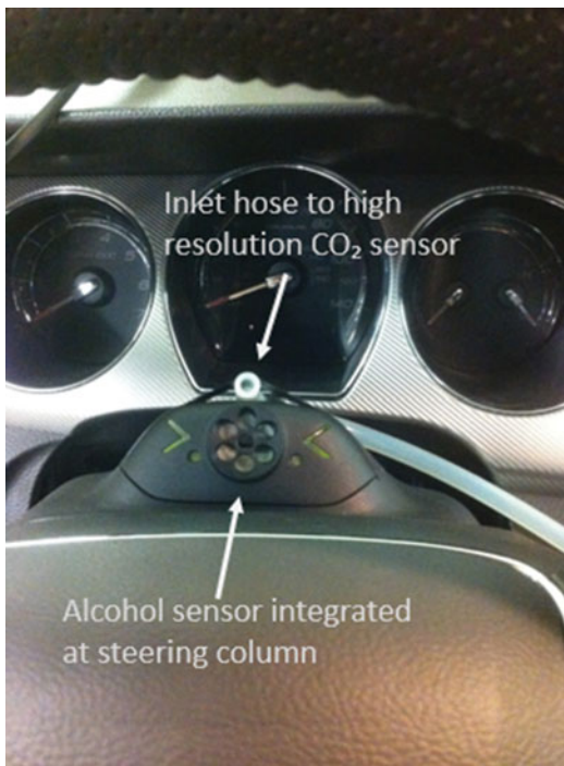
Figure 5. Alcohol sensor integrated at the steering column and inlet hose to high-resolution CO 2 sensor. The integrated alcohol sensor measures both ethanol and CO 2 using 2 optical channels with different wavelengths.
