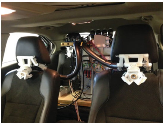
Figure 4. Experimental setup for in-vehicle testing of gas pulses.
