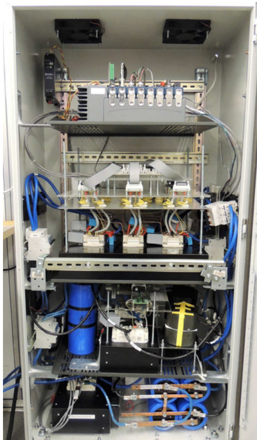
Figure 6.6 Field test arrangement of the WEC to grid interconnection multistage multilevel converter system.
