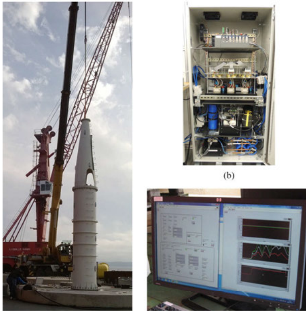
Figure 8.8 Onshore testing of the converter system connected to LPMG output; (a) A crane is used to move the translator up and down to simulate the wave response from the WEC; (b) The power converter systems including rectifier and TLBNPC connected to RL load; (c) LabVIEW GUI showing the converter control response.
