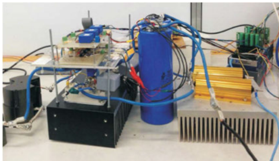
Figure 3.8 Experimental prototype of TLBC with NI CompactRIO – Virtex 5 FPGA and Labview based control system.
