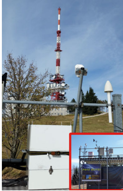
Figure 6. Gaisberg Tower and the X-ray measurement system are shown in the picture. In addition to the white X-ray detector enclosure, vertical E-field antenna, field-mill, and other meteorological instruments are located on the roof of the structure as can be seen in the red-bordered image in bottom-right. The EMC cabinet containing the measuring equipment is inside this structure. The shunts, measuring the current are placed at the tower top.
